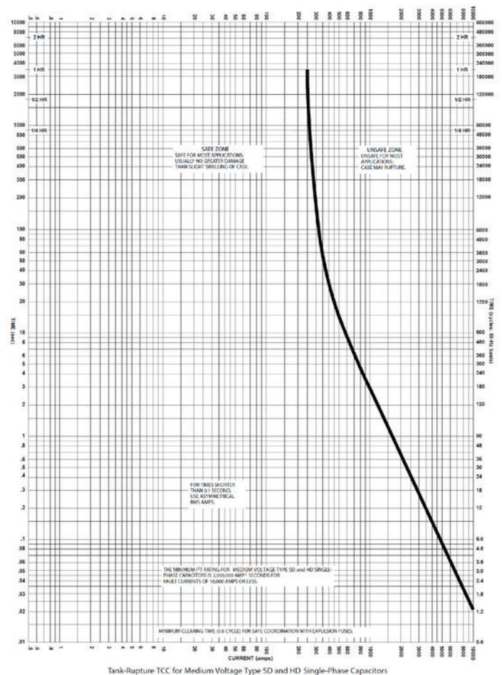
Figure 5. 10 kA Tank Rupture Curve
