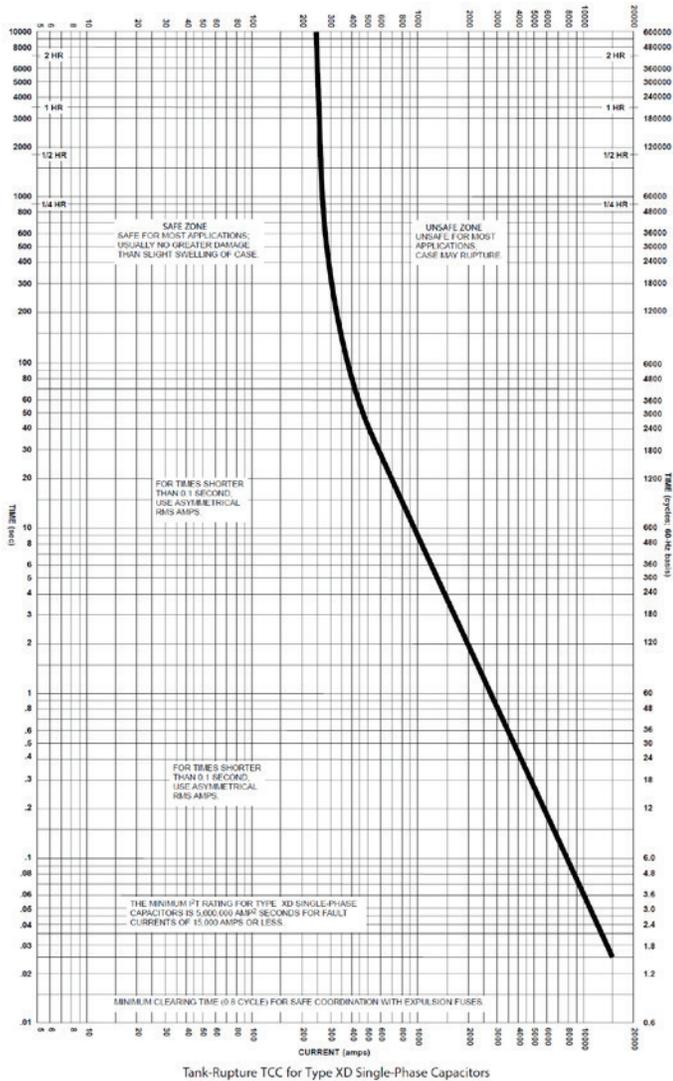
Figure 6. 15 kA Tank Rupture Curve
