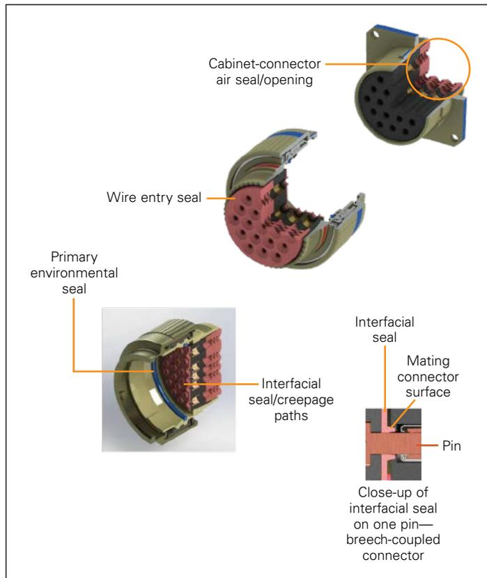
**Figure 1. Location of the environmental seals on the breech-coupled circular connector. Seals on the other circular connectors are located in a similar manner.**
