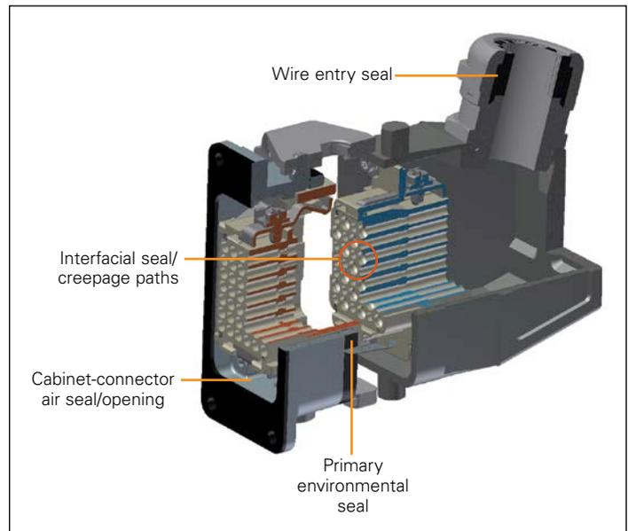
**Figure 2. Location of the environmental seals on the lever-lock rectangular connector.**
