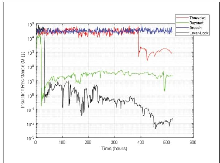
**Figure 4. Insulation resistance over time during humidity testing for each of the four connector types.**
