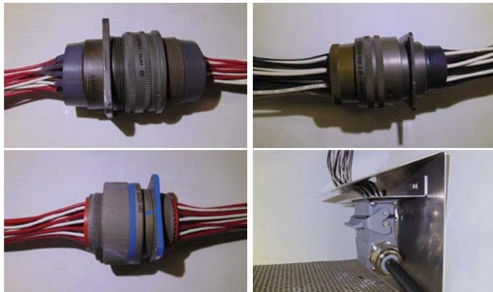
**Figure 3. Preparation of test samples. Upper left: Threaded circular SAE 5015 connector. Upper right: Bayonet circular M26482/SI connector. Lower Left: Breech coupling D38999/IV connector. Lower right: Rectangular lever lock DIN connector.**
