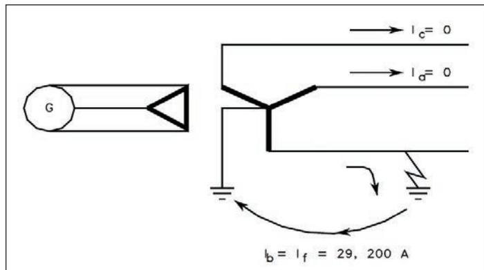
**Figure 4. Ground fault on a solidly grounded system**
