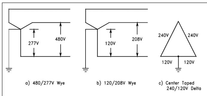
**Figure 6. Solidly grounded systems (industrial/commercial)**
