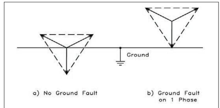
**Figure 3. Voltages during ground fault**
