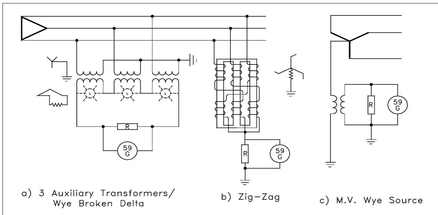
**Figure 11. Grounding transformers**
