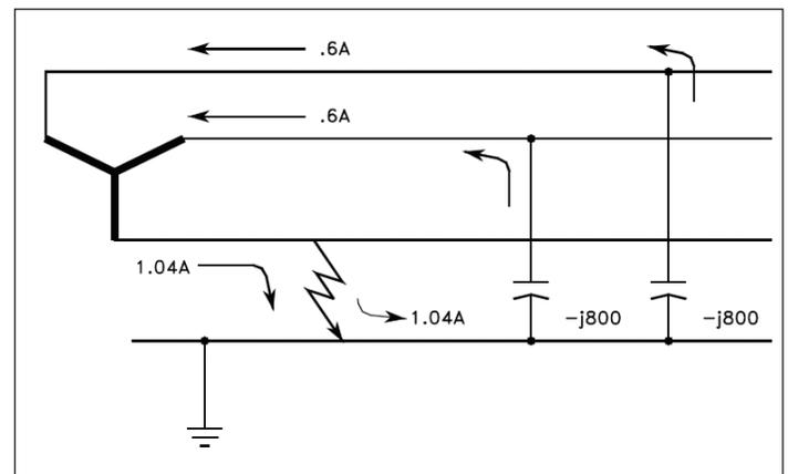
**Figure 2. Ground faults on ungrounded systems**
