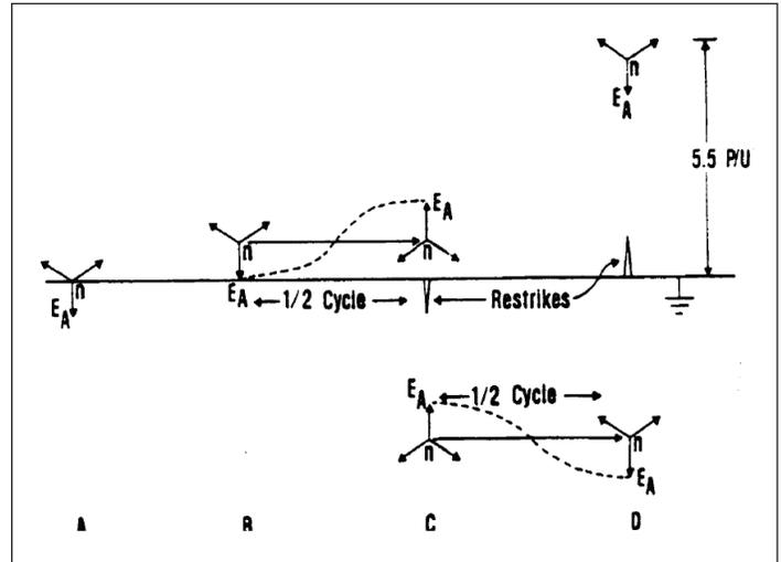
**Figure 8. Transient overvoltages from restriking ground fault**
