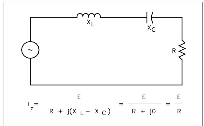
**Figure 7. Series resonant circuit (when  $X_L = X_C$ )**
