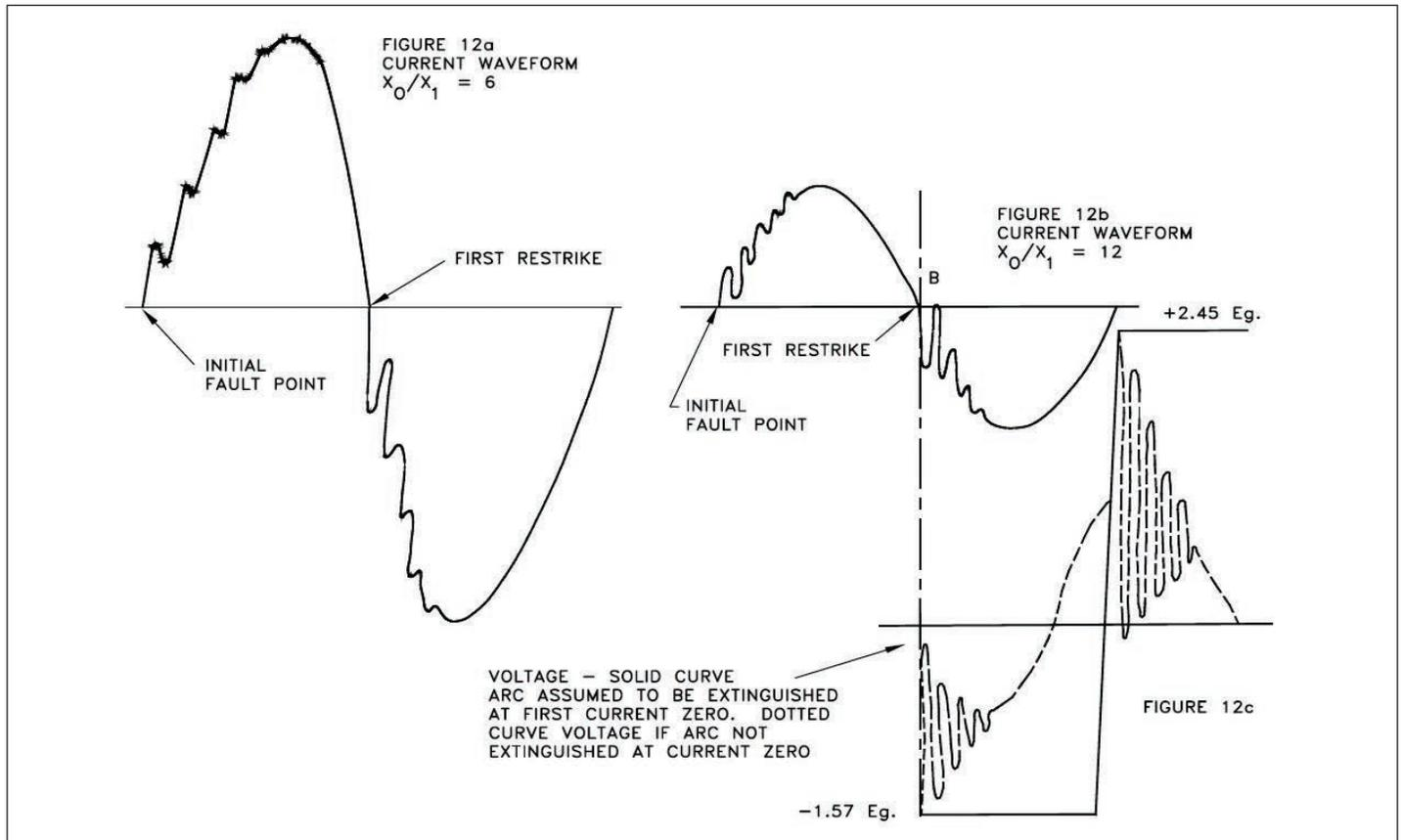
Figure 12. The effect of grounding impedance on transient overvoltage
