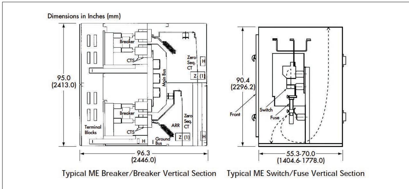
**Figure 2. Section views of typical feeder devices**
