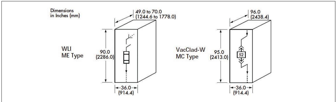
**Figure 1. Typical one-lines and elevations for single indoor structures**
