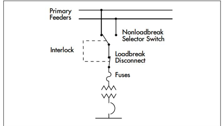
**Figure 5. Fused selector switch in one structure**
