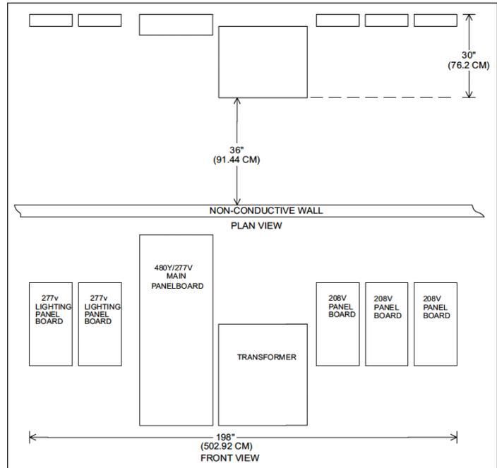
**Figure 1. Conventional panelboard/transformer room layout**
