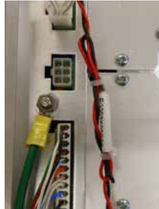
Figure 10. Eliminate the excess power cord length.
