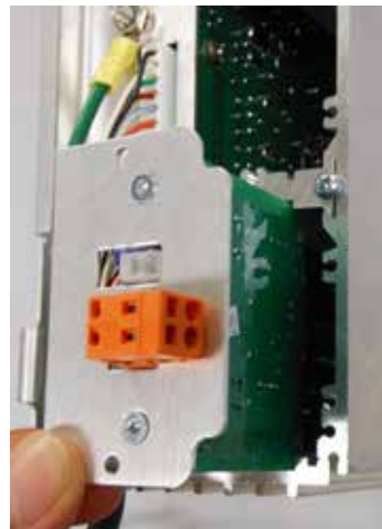
Figure 6. Inserting the DC power module into the accessories slot in a single-phase control.
