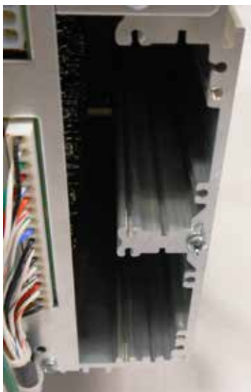
Figure 5. Aluminum card-support bar secured with 0.25" screw.
