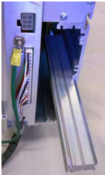
Figure 4. Installing aluminum card-support bar into accessories slot.
