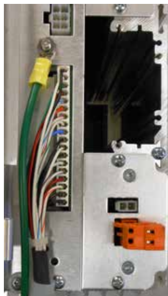
Figure 7. Securing the DC power module with screws into the accessories slot of the main control panel.
