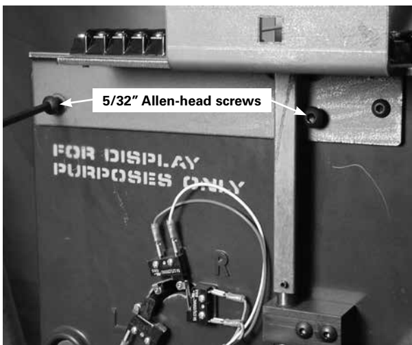
Figure 19. Terminal board bracket fastening
