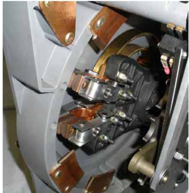
Figure 4. Main movable contacts in number 1 stationary position.
