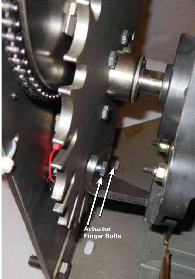
Figure 25. Installing the actuator finger.
