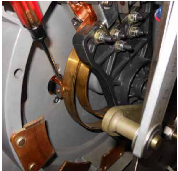
Figure 15. Inserting the outer contact ring between the button contacts.
