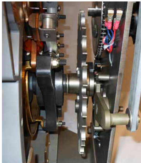
Figure 20. Geneva gear rotating freely on main shaft.
