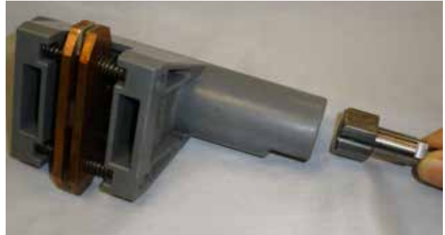
Figure 12. The actuator shaft removed from the reversing movable contact assembly.
