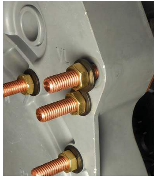
Figure 7. VL reversing stationary hardware
