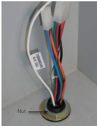
Figure 33. Securing the pigtail with a nut and washer.
