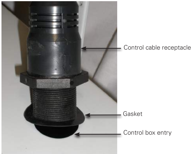
Figure 17. Installation of control cable.
