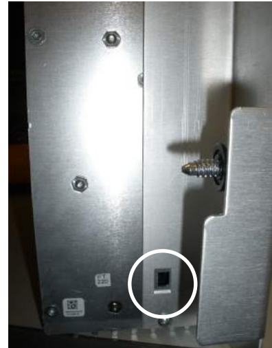
Figure 26. Neutral light source switch.
