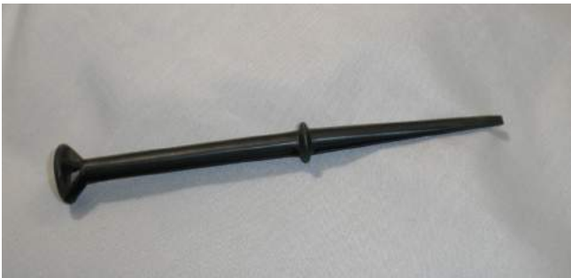
Figure 21. Wire insertion tool.
