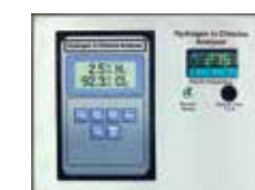
Hydrogen and chlorine analysers
