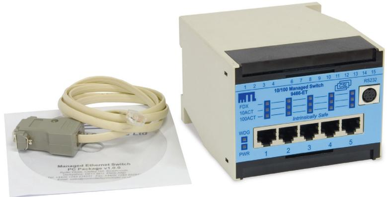
The 9466-ET 10/100Mbps, Layer 2, Ethernet switch allows the interconnection of MTL 9460-ET range networking modules via its 5 ports. It also enables an Ethernet network to cover a greater distance using either Cat5e cable or fibre-optic for longer spans. This capability is due to the low latency 'store and forward' mechanism integral to the switch, which ensures that the stringent timing associated with Ethernet is maintained.
