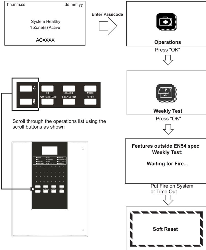
Figure 23. Operations (Weekly Test) screen
