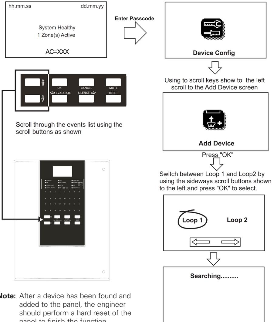
**Figure 40. Device Config (Add Device) screen**
