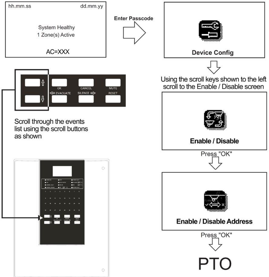
**Figure 42. Device Config (Enable/Disable Address) screen**
