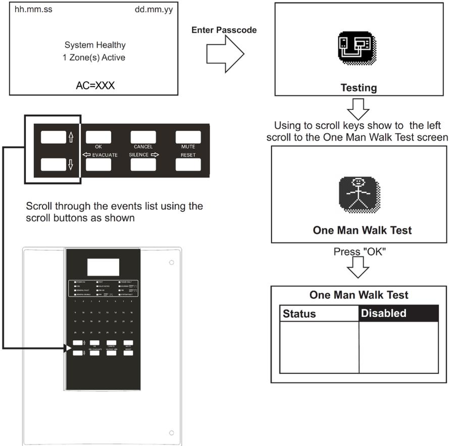
**Figure 37. Testing (One Man Walk Test) screen**
