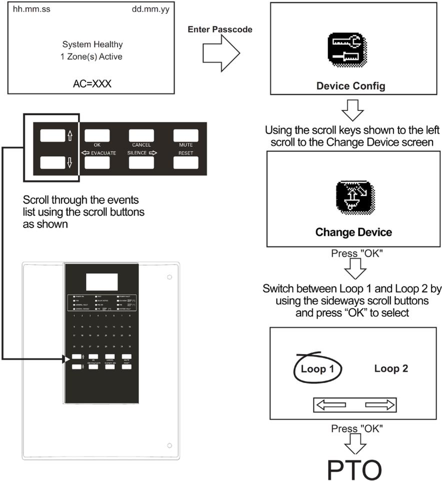
Figure 47. Device Config (Change Device) screen
