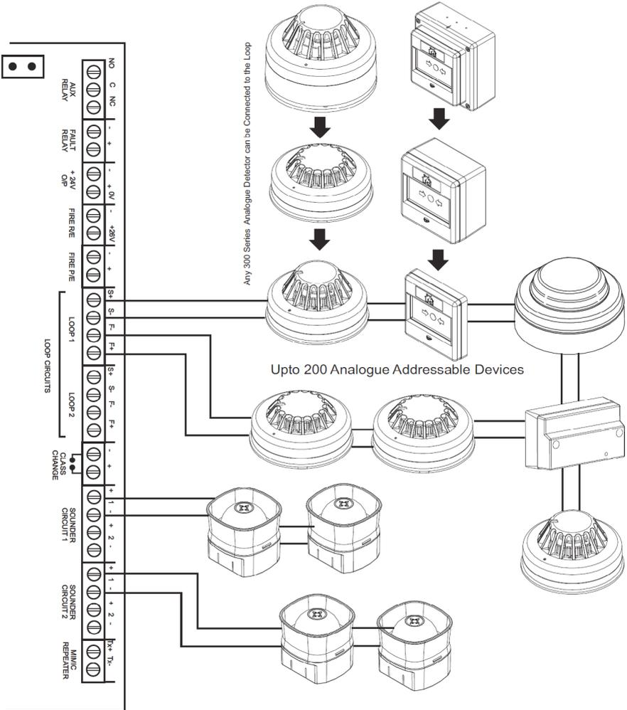
Figure 3. Typical System Wiring diagram
