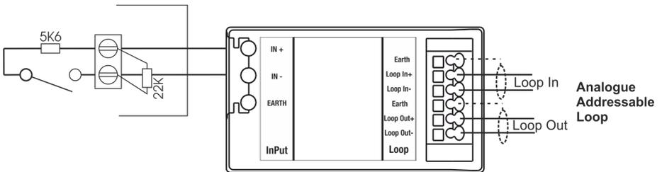
**Figure 64. Standard connections**
