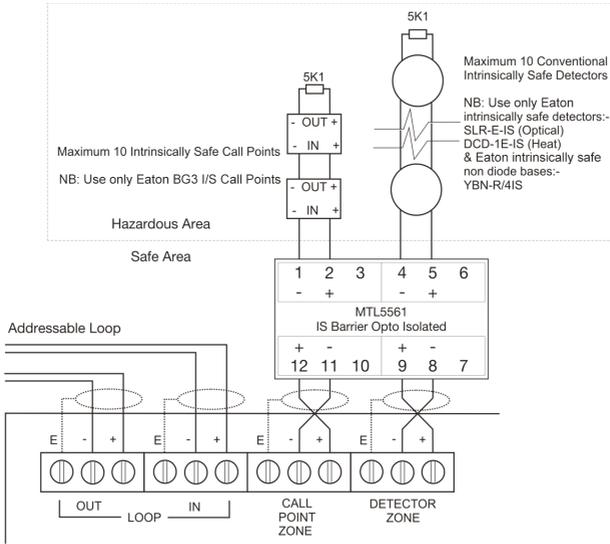
**Figure 59. Standard connections**
