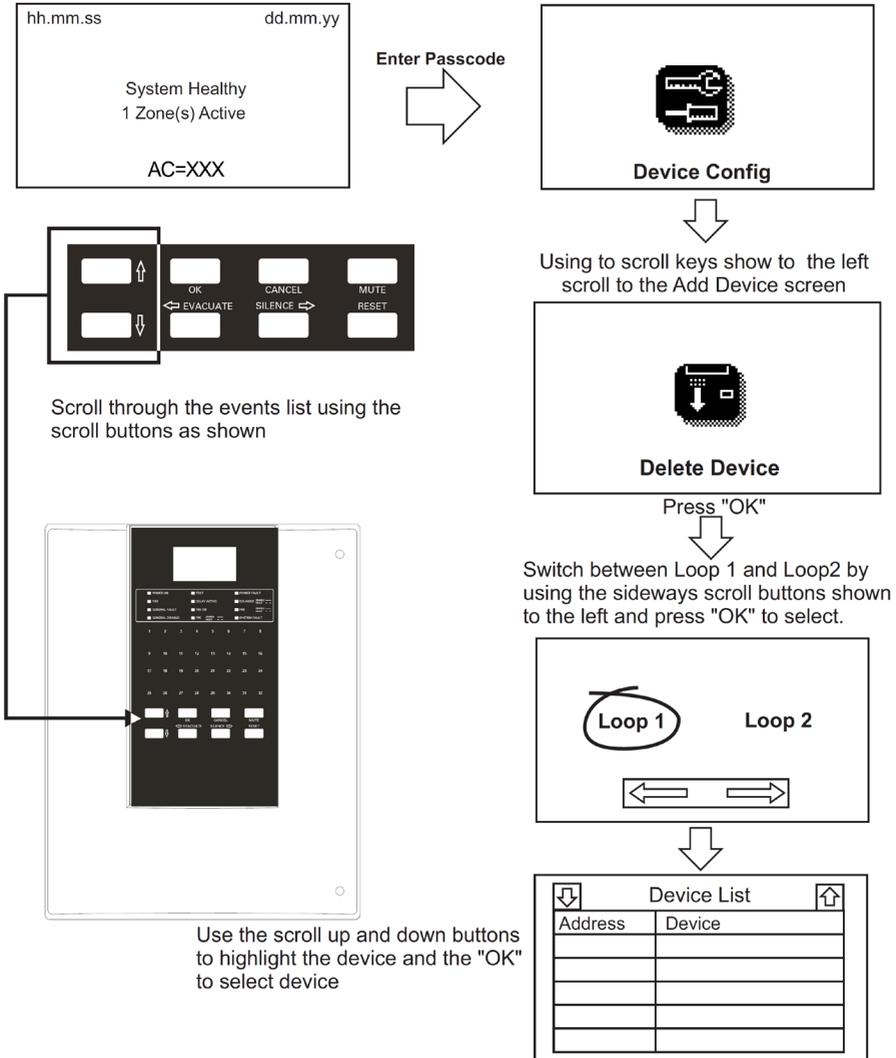
Figure 41. Device Config (Delete Device) screen
