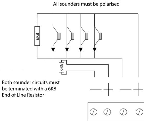
**Figure 1. Typical Sounder circuit**
