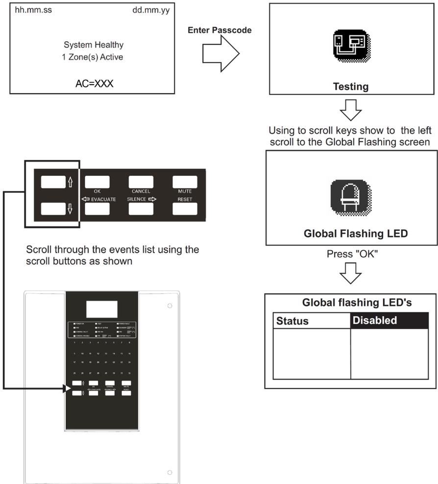
**Figure 38. Testing (Global Flashing LED) screen**
