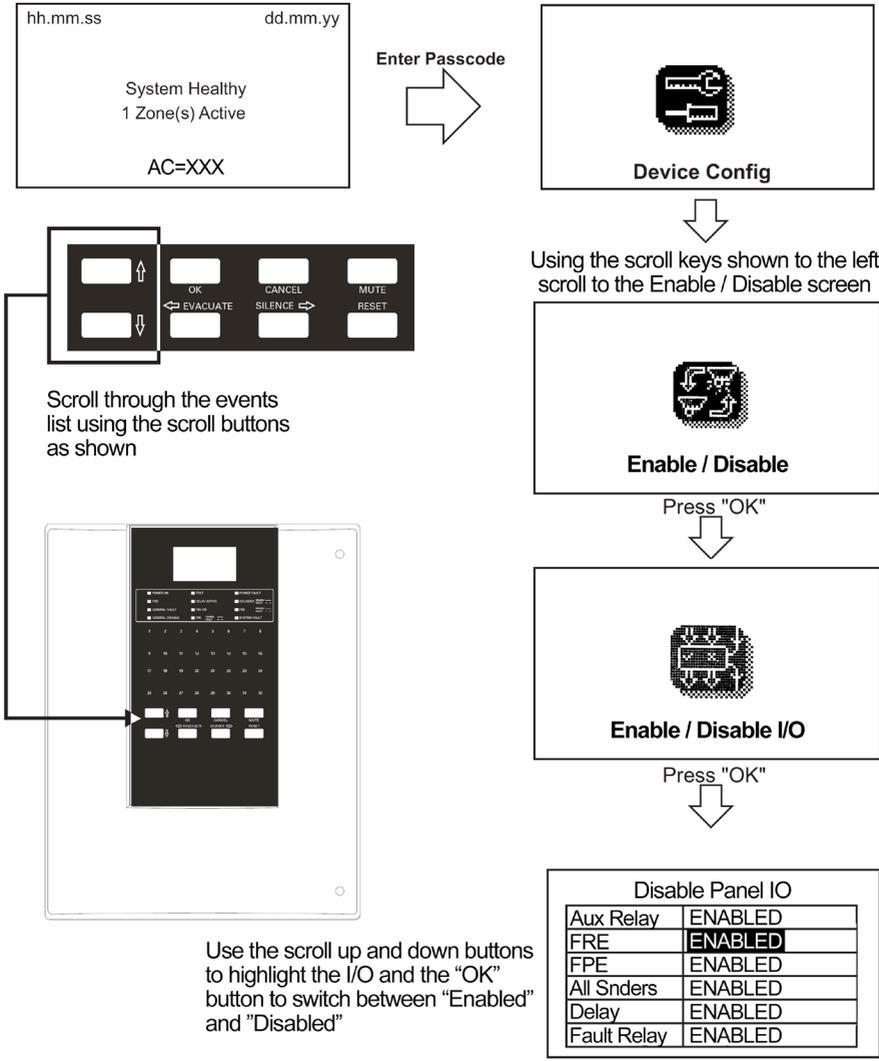
Figure 45. Device Config (Enable/Disable I/O) screen
