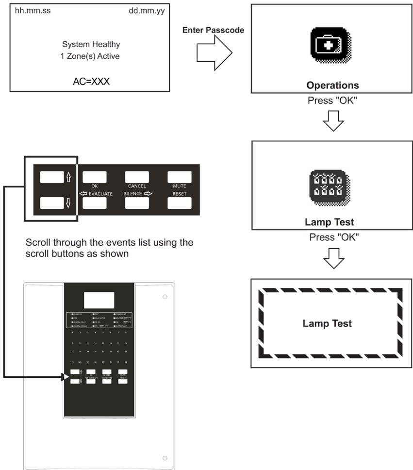
**Figure 22. Operations (Lamp Test) screen**
