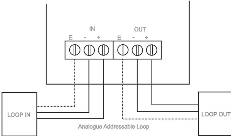
**Figure 53. Loop powered beacon**
