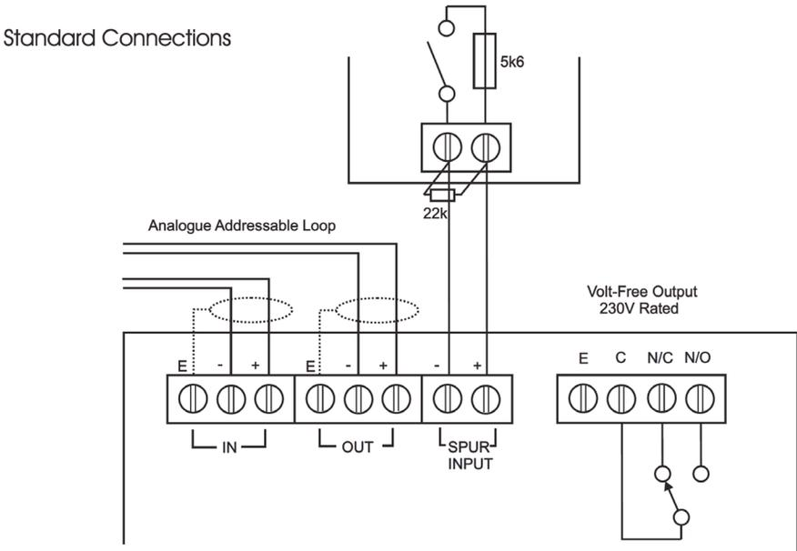
Figure 57. 1 Way Input Output Unit
