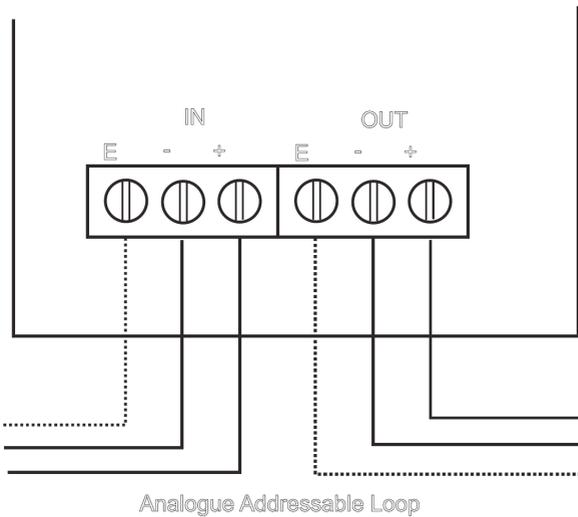
**Figure 54. Internal Wall Sounder**
