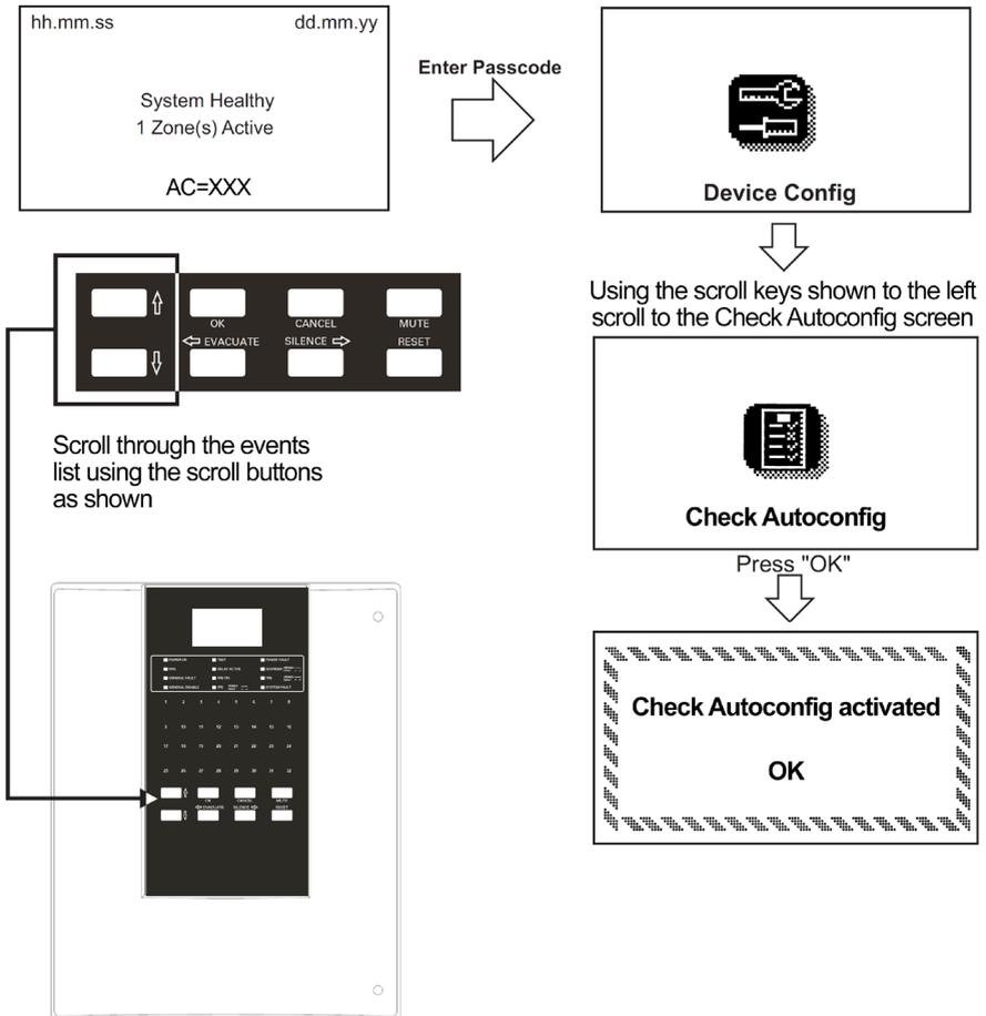
Figure 46. Device Config (Check Autoconfig) screen
