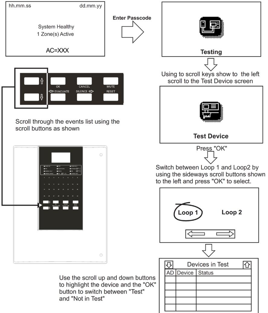
Figure 34. Testing (Test Device) screen
