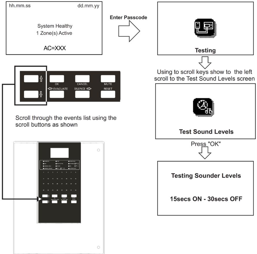
**Figure 36. Testing (Test Sound Levels) screen**
