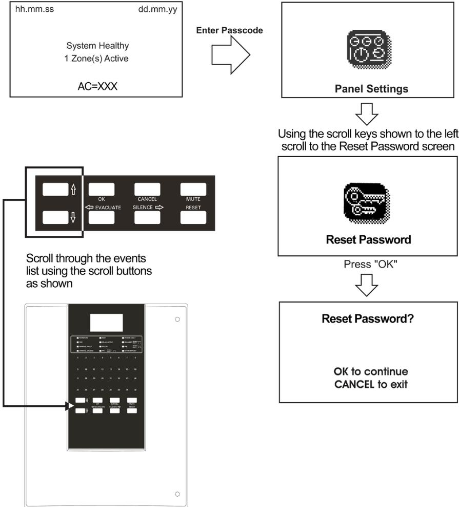
Figure 29. Panel Settings (Reset Password) screen
