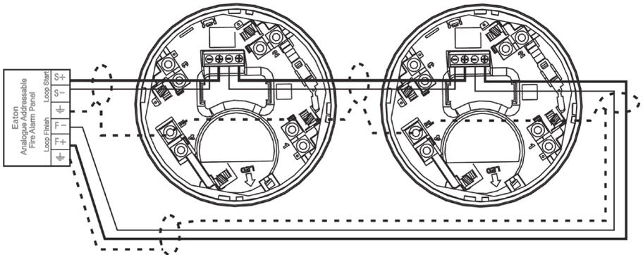
**Figure 52. Base sounder and sounder beacon base wiring**
