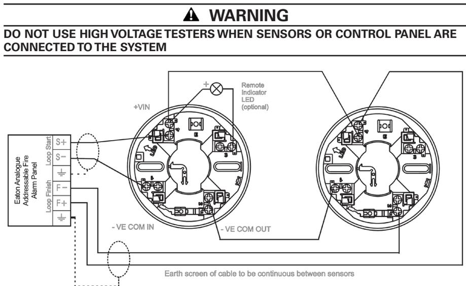
**Figure 50. Wiring Diagram for Sensor Base**
