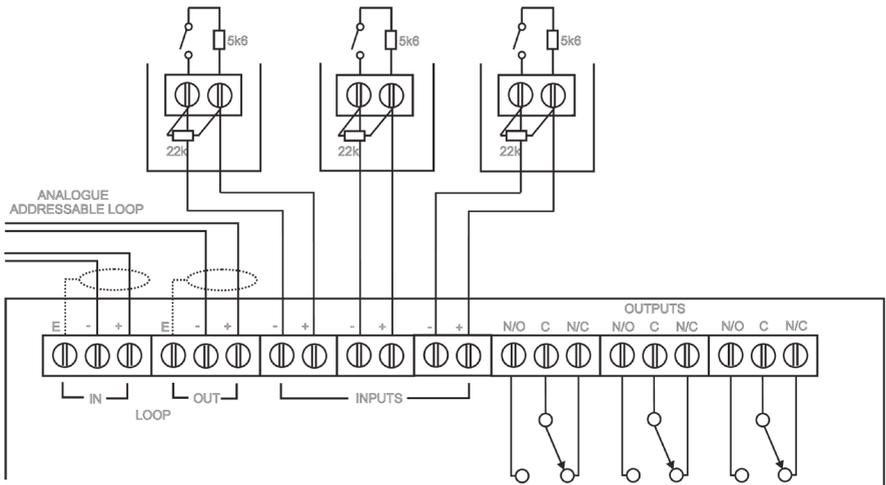
**Figure 56. Wiring for 3 way Input/Output unit**
