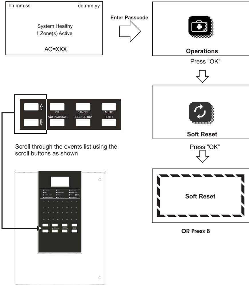
Figure 19. Operations (Soft Reset) screen
