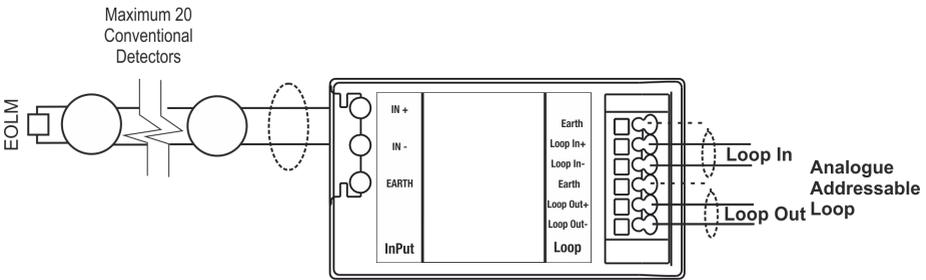
**Figure 63. Standard connections**
