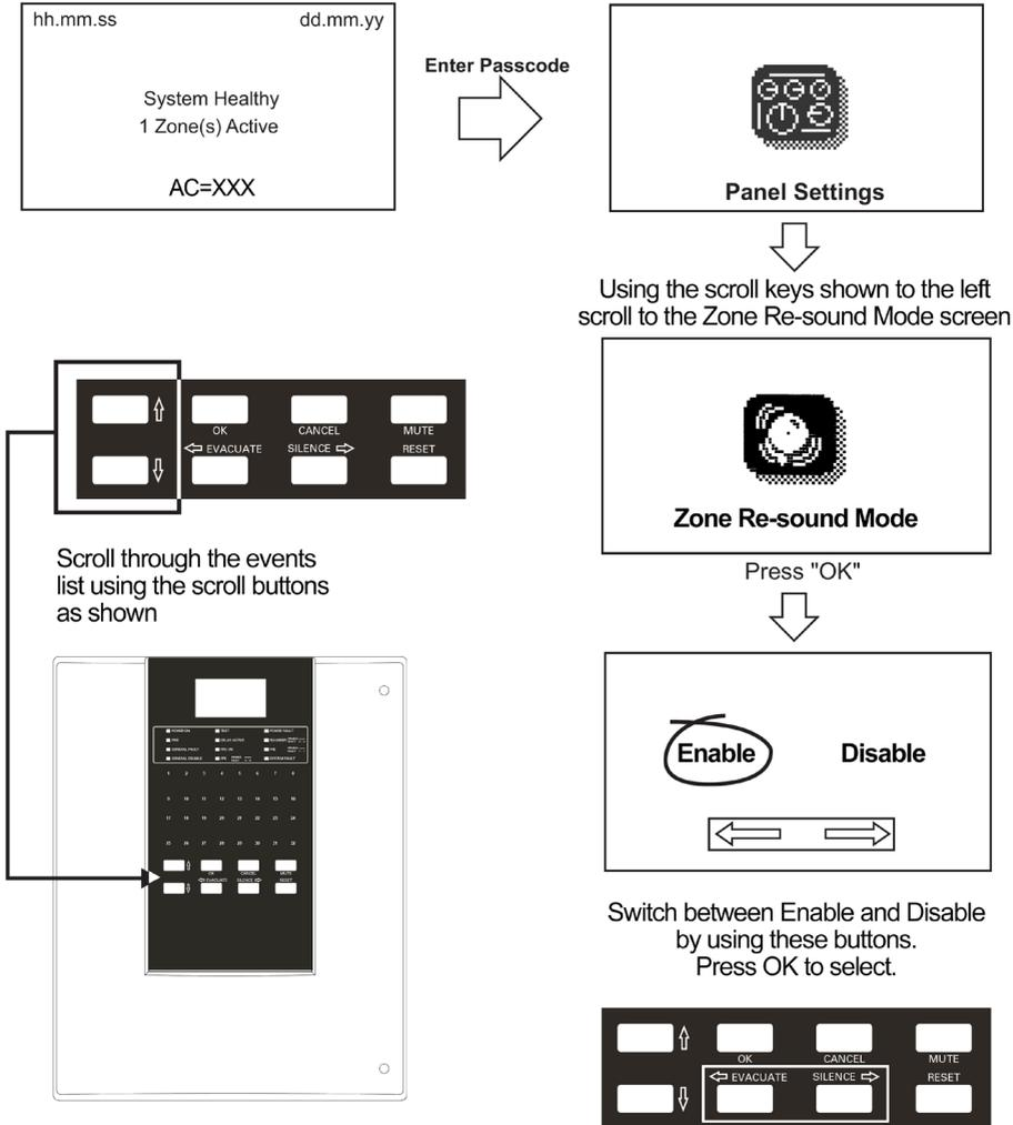
Figure 27. Panel Settings (Zone Re-sound Mode) screen
