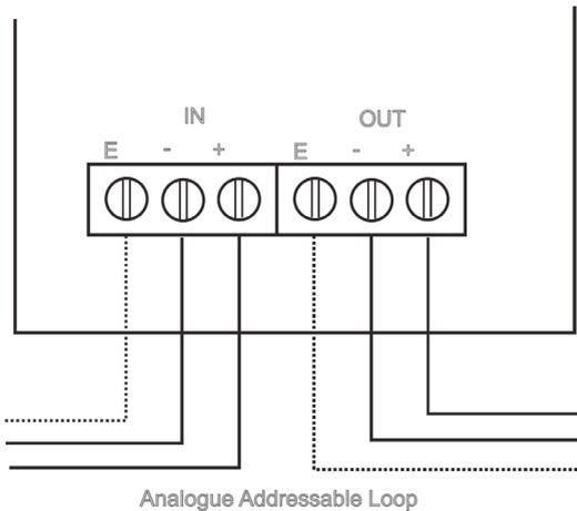
**Figure 55. II Sounder Wiring**
