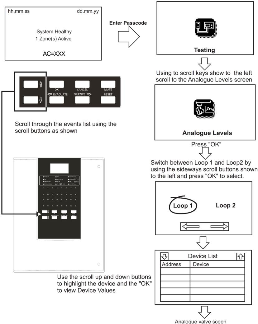
**Figure 39. Testing (Analogue Levels)**
