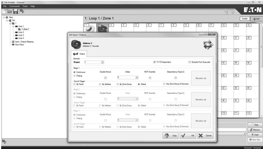
Figure 6. Device Outputs
