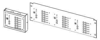
FC6 and FC18 Interface are designed to work with the Eaton range of analogue fire alarm control panels, providing the capability to control and display the status of AHU fans.
