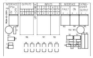
This board can be connected to an Extinguishing system as well as a Fire Brigade Control Panel. This board has been tested and approved in according with DIN14661 and DIN 14675.
