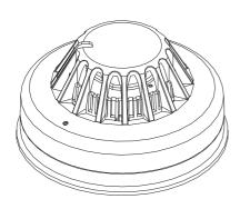
**Addressable Heat Sensor,** this is suitable for dusty environments or environments where smoke is likely to be present under normal operating conditions. The heat detectore can be programmed to operate in A1R,BS or CS mode of operation depending on the required application and sensitivity requirements.
