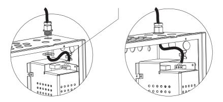
**Note:** The mains cable tail ends must be insulated to prevent dangerous conditions arising in the event of accidental switching on of the mains supply.
