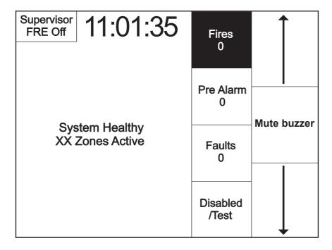
The Touch Screen is a multi-function display consisting 320x240 dots featuring high intensity backlighting. In normal operation, the display indicates as above with the backlighting off.
