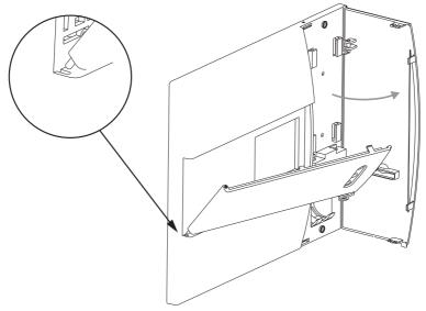
Insert the bottom peg of the hinged cover into the panel as shown and close the hinged cover followed by the printer door. Next from the back of the panel insert second peg though the hole shown below and push into the hinged cover.
