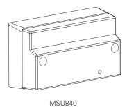
MSU840 accepts a zone of conventional detectors plus an unlimited number of callpoints which can be connected to the same input as the detectors or a separate callpoint input if required. It also has a 24V 1A rated relay output, and a facility to connect a power supply, which can then be monitored for fault. In addition it has the facility to connect two circuits of conventional polarised sounders, which are monitored by means of an end of line resistor and powered in alarm conditions from
