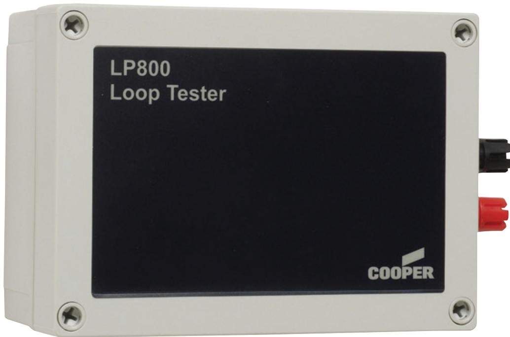
The loop tester kit (LP800KIT) is a hardware / software combination that can be used to test, commission and fault find a loop of up to 200 intelligent addressable devices (sensors, sounders, ancillary devices) without having to connect the loop to Eaton's intelligent addressable control panel.
