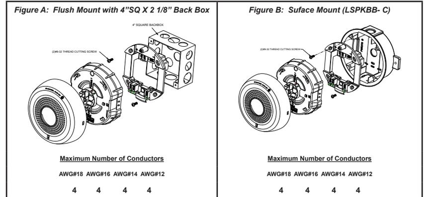
**CAUTION:** Check that the installed product will have sufficient clearance and wiring room prior to installing backboxes and conduit, especially if sheathed multiconductor cable or 3/4-inch conduit fittings are used.
