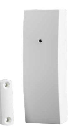
Grade2, radio door contact with configurable second radio channel with wired inputs. For use with HUA (PA), door contact, key switch or other voltage free device. Compact unit with replaceable CR2 lithium battery.
