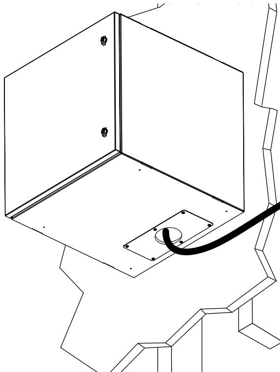
**Note:** To maintain a NEMA rating, use sealed fittings in the cutouts when connecting to conduit.
