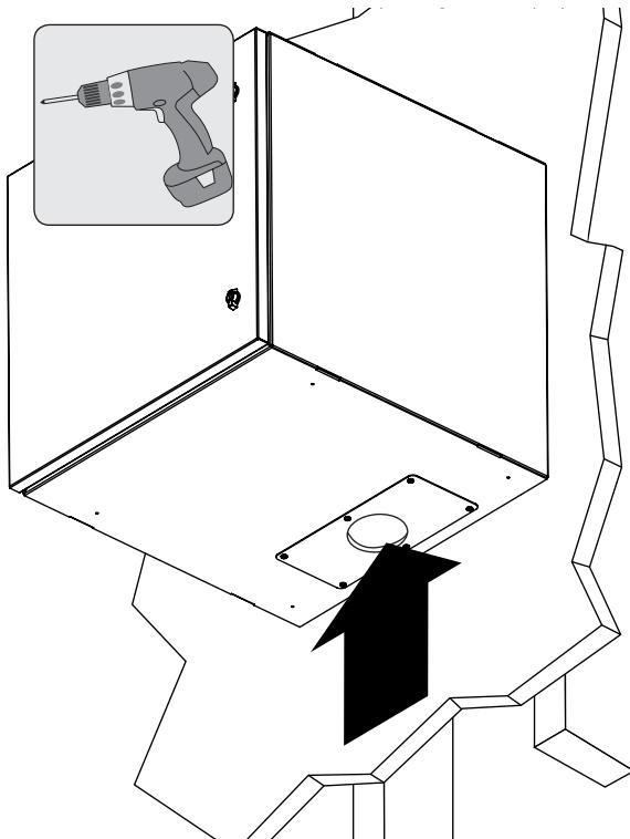
**Note:** This conduit cover supports a maximum Conduit Trade Size 2 with 2.5" hole.
