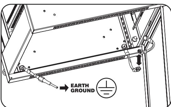
**Warning:** Attach each enclosure to earth ground separately. Do not use the enclosure without an earth ground connection.
