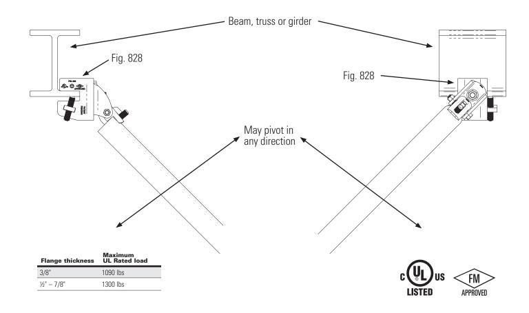
**Installation Instructions:** Slide the Fig. 828 on the flange of the beam, truss, or girder. Be sure the attachment is fully engaged to the rear of the opening. Tighten the cone point set screws until the heads break off. Remove the flange nut from the carriage bolt. Install a TOLCO swivel fitting (Fig, 909, 910, 980, \*986). Use flange nut to secure the swivel fitting.
