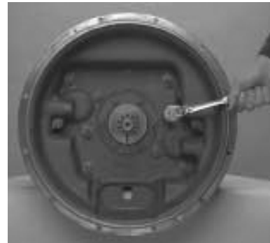
Recommended Clutch Housing Tightening Pattern
