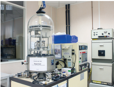
Vacuum bell for robotic operating testing -170°C/+200°C temperature gradient
