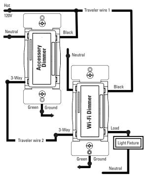
For multi-location applications (3-way or 4-way), the **Accessory Dimmer (EWACD)** or a regular 3-way switch with one **Wi-Fi Smart Dimmer (EWFD30)** can be used.
