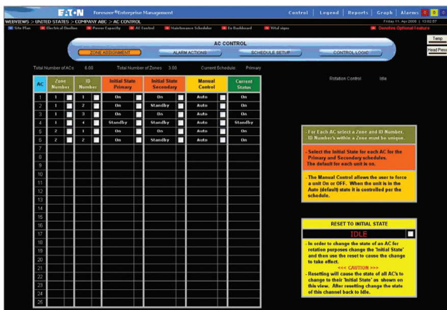
Figure 16: AC Control Zone Assignment View
