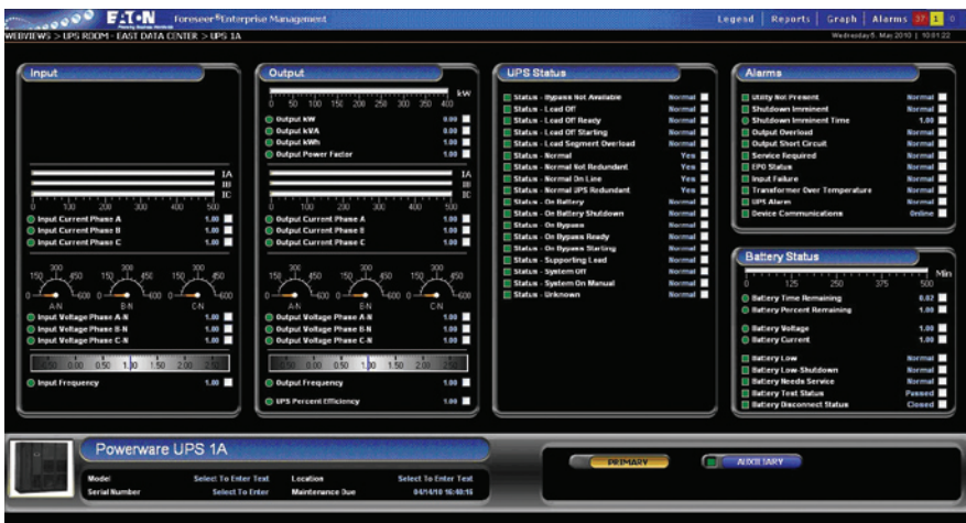
Figure 12: This Data Center UPS equipment view example displays at-a-glance the most critical data coming from a UPS system. Input, output, status and alarms along with battery information provide a great inner view into the UPSs overall performance. Note that fields for system location and e.g. battery maintenance schedule can be made available automatically.
