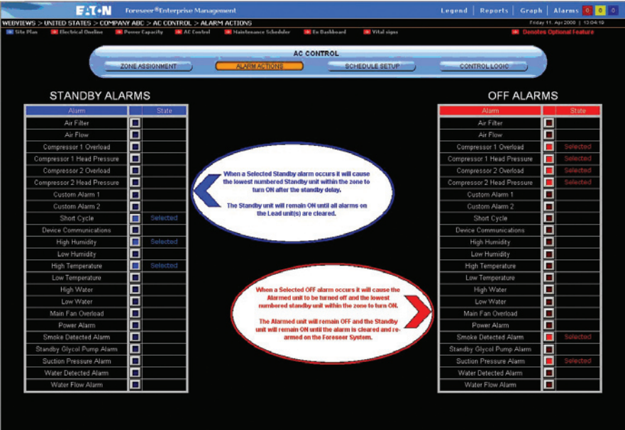
Figure 13: AC Control Alarm Actions View
