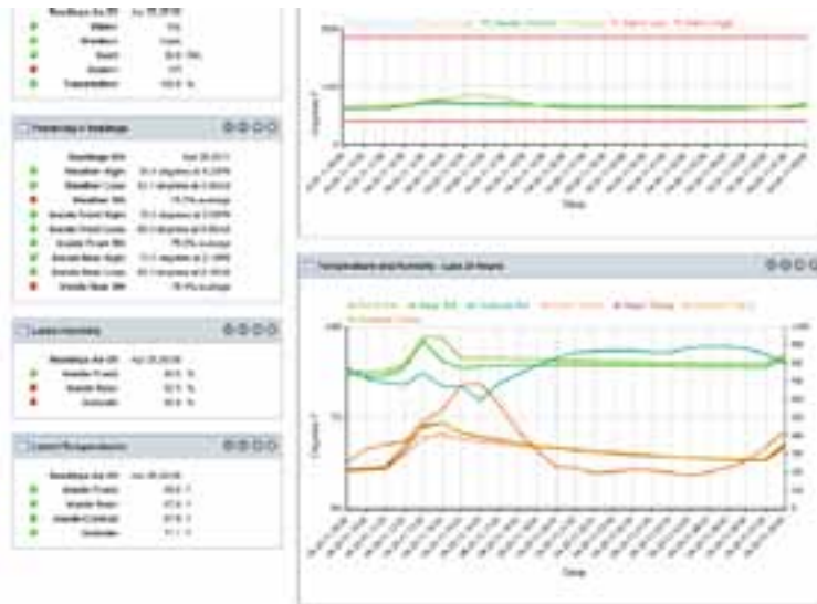
This sampling of data shows the proper difference in temperature and humidity in an outdoor bus duct
