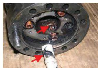
ESP ground fault failure in wye point
