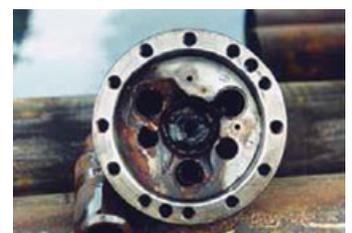
ESP ground fault failure tandem section
