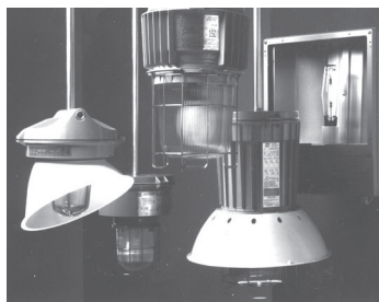
Eaton's Crouse-Hinds luminaires are certified as ExnR "restricted breathing" for Division 2 locations
