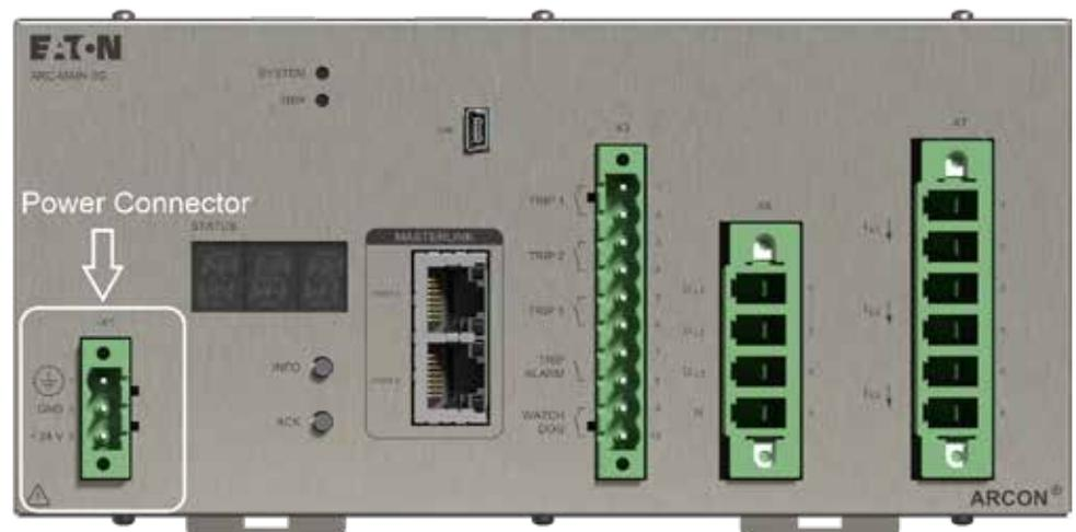
Figure 3.3 Master MAIN – Power connector
