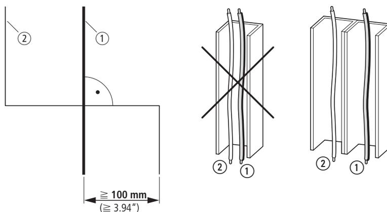
Figure 113: Laying of signal and power cables
