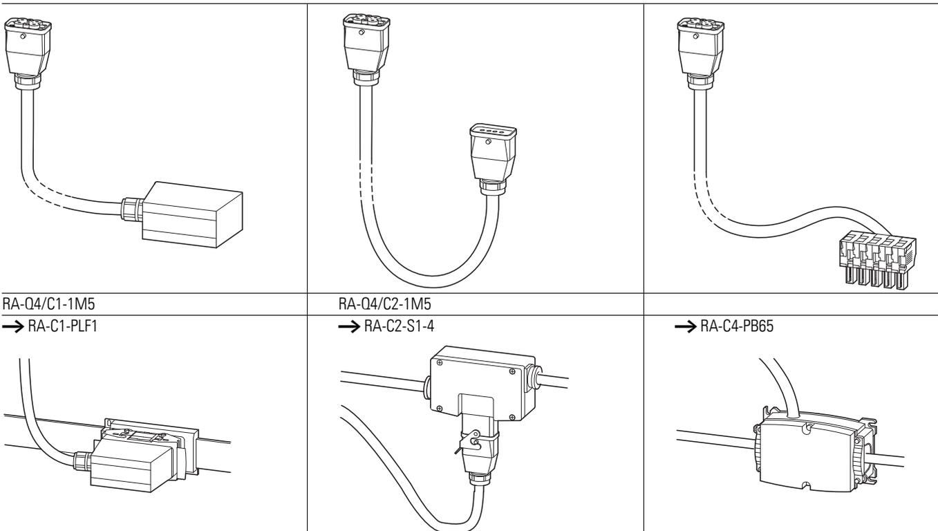
After installing the power bus outgoers (RA-C1-PLF1, RA-C2-S1-4, RA-C4-PB65) you can connect the Rapid Link module (RAMO5/RASP) to the power plug using the assigned power adaptor cables.
