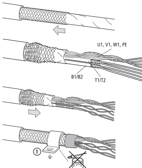
Figure 67: EMC-compliant connection of the screened motor cable
