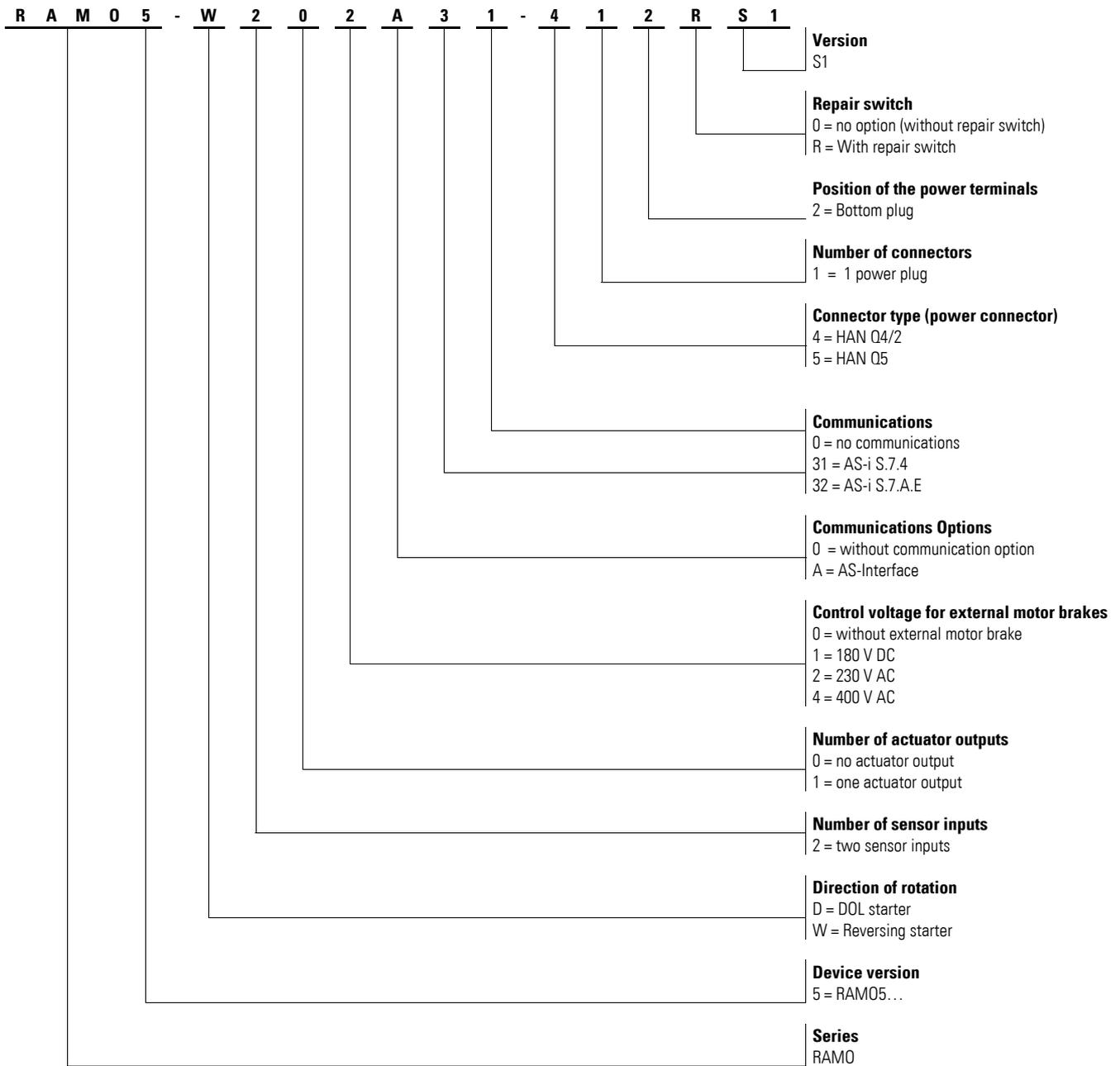
Figure 5: Key to part numbers of RAMO5 motor starter
