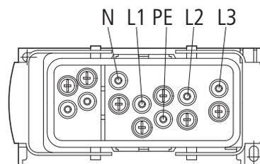
Figure 52: Pin assignment for flexible busbar junction RA-C1-PLF1
