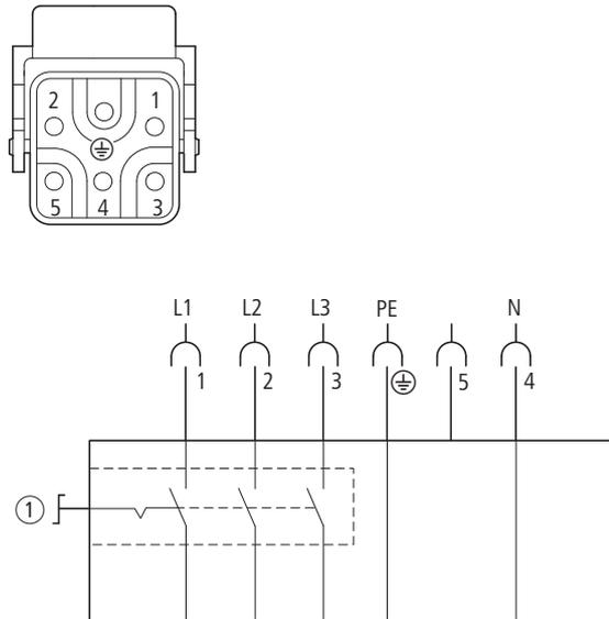
Figure 11: Repair and maintenance switch in position 0 = OFF
