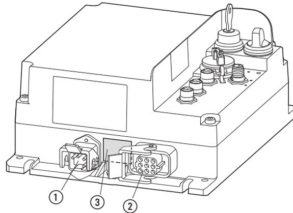
Figure 14: Connections in RAMO5 power section
