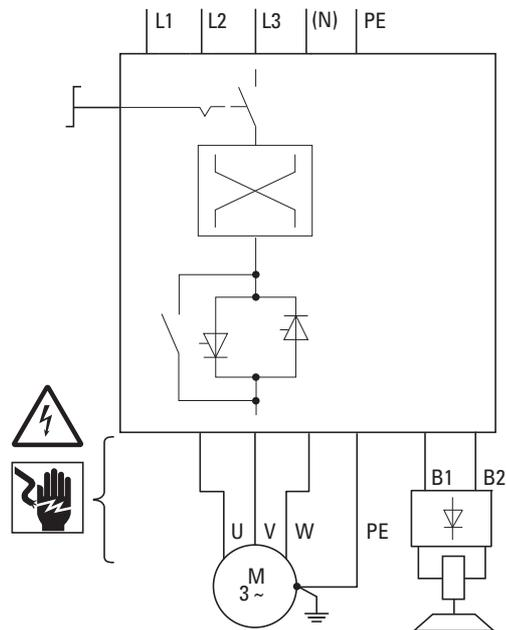
Figure 79: Reversing starter with repair and maintenance switch and brake control RAMO5-Wxx1(2)(4).....RS1
