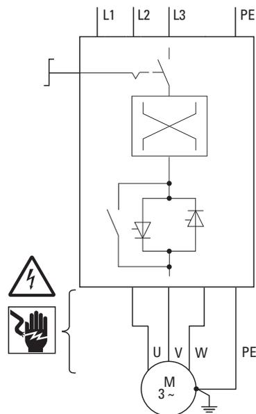
Figure 78: Reversing starter with repair and maintenance switch RAMO5-W...-...RS1
