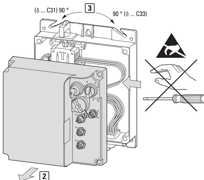
Figure 45: Example: Lift off the housing cover on a RASP5
