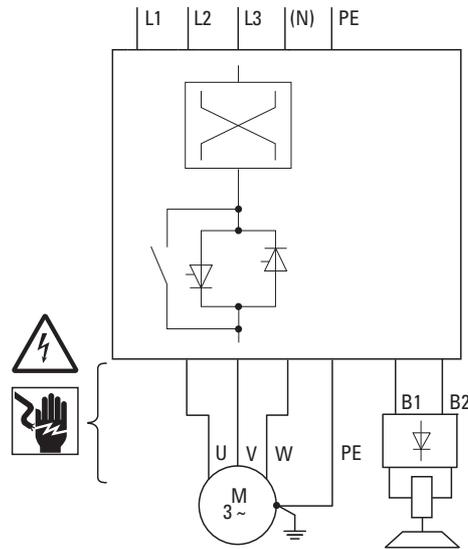
Figure 77: Reversing starter with brake control RAMO5-Wxx1(2)(4)...-...0S1
