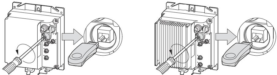
Figure 100: Parameterization via Bluetooth stick DX-COM-STICK-KIT
