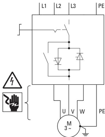
Figure 74: Direct starter with repair and maintenance switch RAMO5-D...RS1
