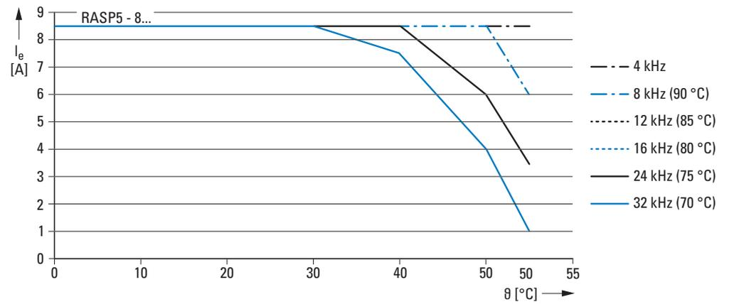
Figure 93:  $f_{PWM}$  = 4 - 32 kHz for RASP5-8...
