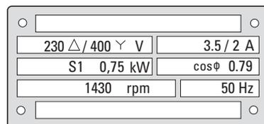
Figure 28: Example of a motor ratings plate
