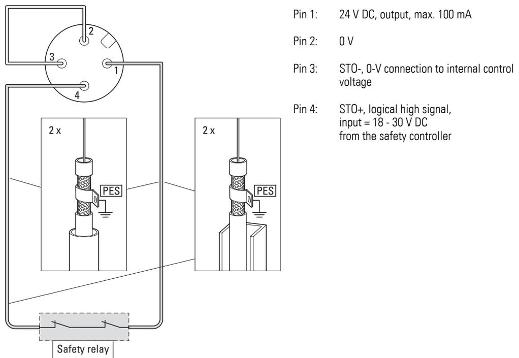
Figure 20: STO installation with internal control voltage
