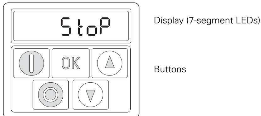
Figure 106: View of the DX-KEY-LED2 control unit
