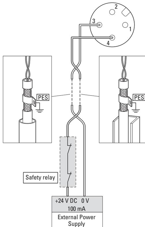
Pin 3: STO-, 0-V connection to internal control voltage
