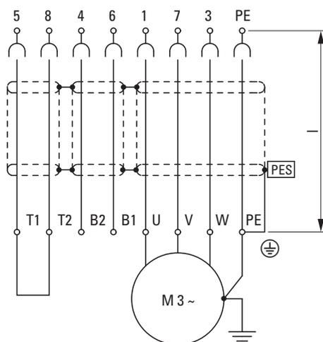
Figure 66: Shielded motor cable for RASP5.
