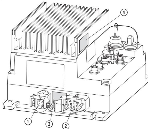
Figure 80: Connections in RASP5 power section and hazard warnings
