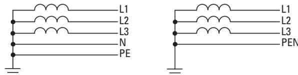
Figure 16: AC power networks with grounded center point (TN/TT networks)
