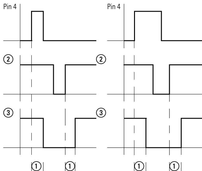
Figure 31: Examples: Edge-controlled quick stop in automatic mode (pin 4 = I1)
