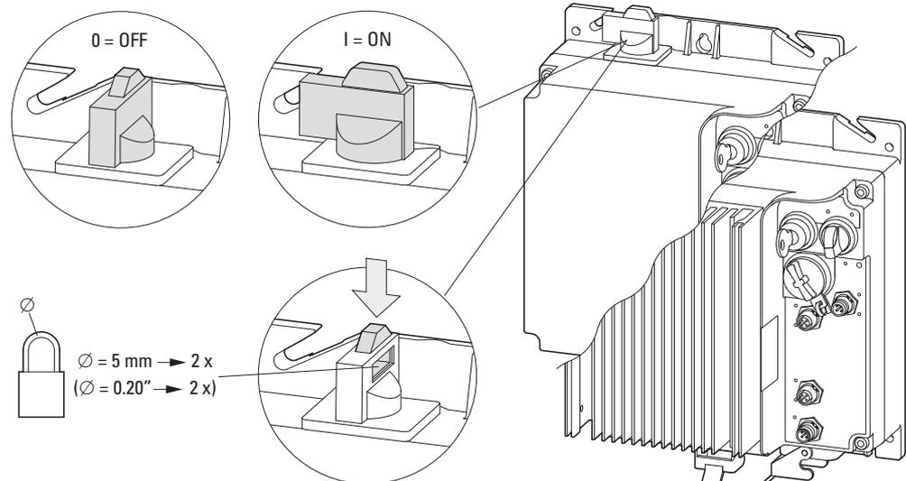
Figure 13: RASP5 with repair and maintenance switch
