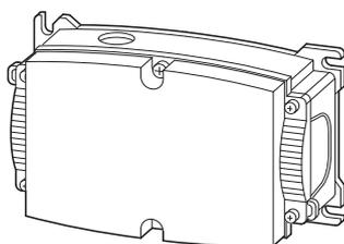
Figure 55: RA-C4-PB65 round cable junction (power box)
