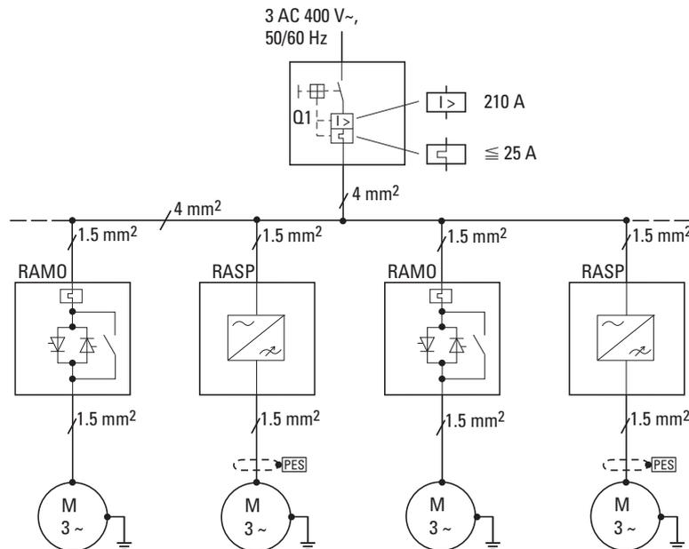
Figure 17: Sample configuration of a Rapid Link system with RAMO5 and RASP5 units
