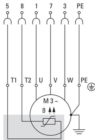
Figure 64: General motor connection with thermistor, motor feeder plug and motor cable monitoring
