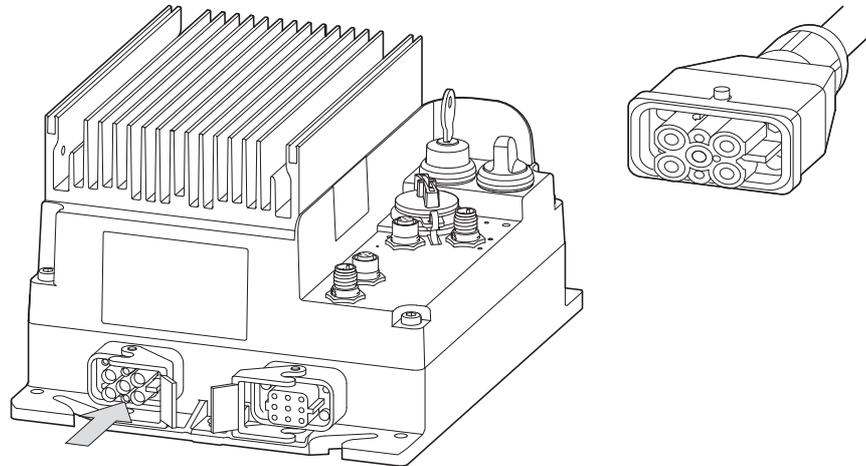
Figure 61: Energy connector RA-Q4...
