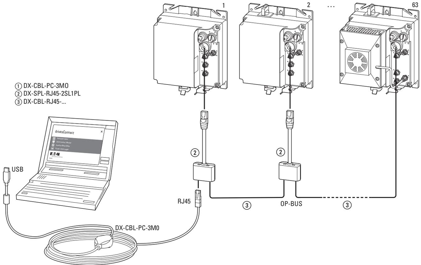
Figure 114: System configuration for system bus
