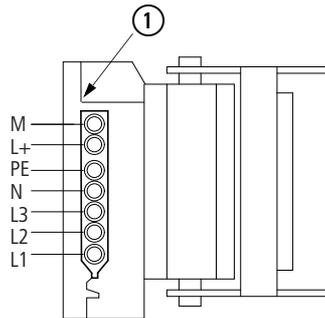
Figure 48: Keying on RA-C1-7... flexible busbar
