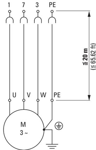
Figure 63: General motor connection with motor feeder plug and motor cable monitoring
