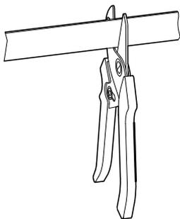
Figure 50: RA-C1-CUT hand ribbon cable cutter
