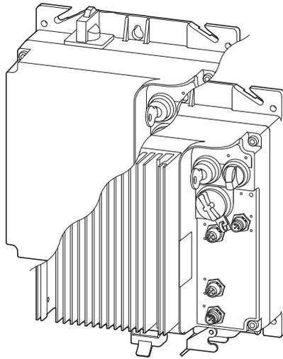
Figure 23: Terminal sockets for I1 and I2 sensor inputs
