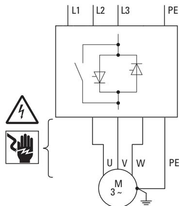
Figure 72: Direct starter RAMO5-D...-...0S1 (without repair switch)
