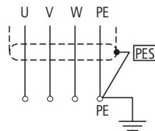
Figure 69: Connecting a screen braid (PES) to the motor terminal box
