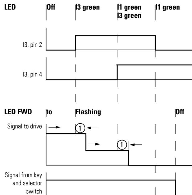
Figure 98: Interlocked manual operation with creep speed
