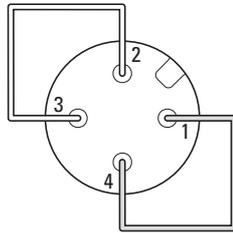
Figure 22: STO control signal terminals (direct enable)
