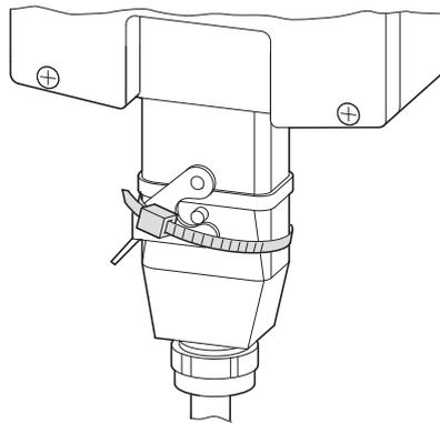
Figure 70: Securing the motor outlet plug by cable ties
