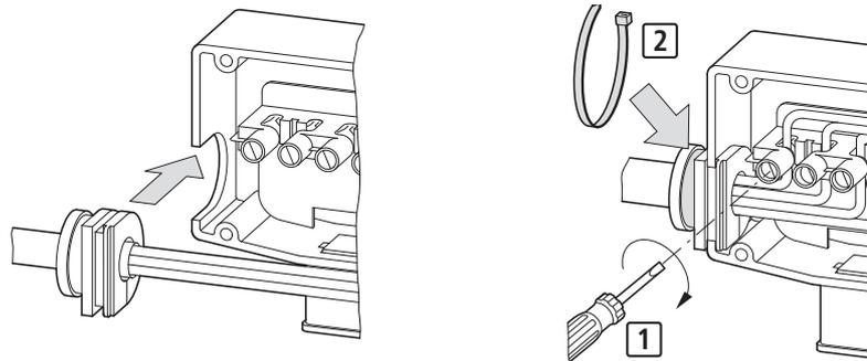
Figure 54: Round cable connection
