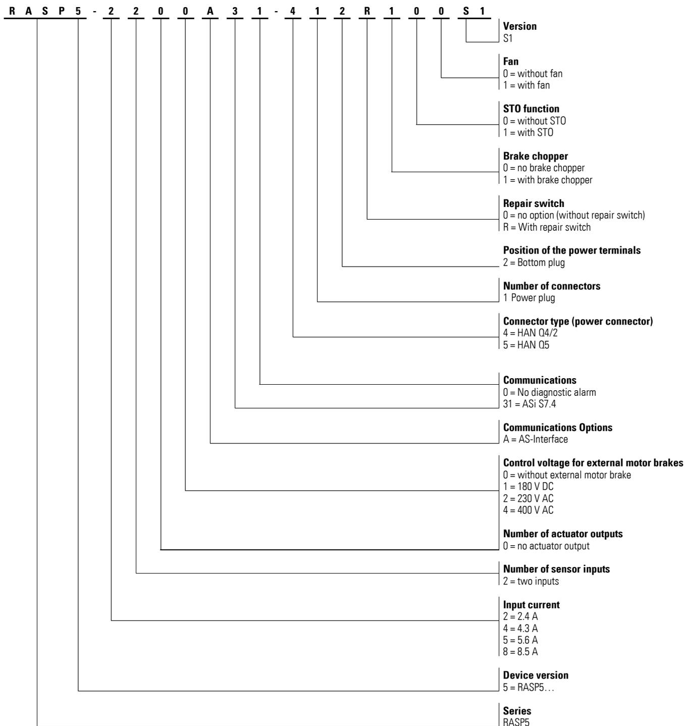
Figure 6: Key to parts numbers of the RASP speed controller
