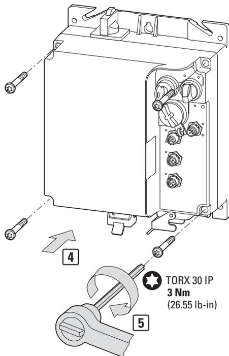
Figure 47: Fastening the M32 screw-on cover
