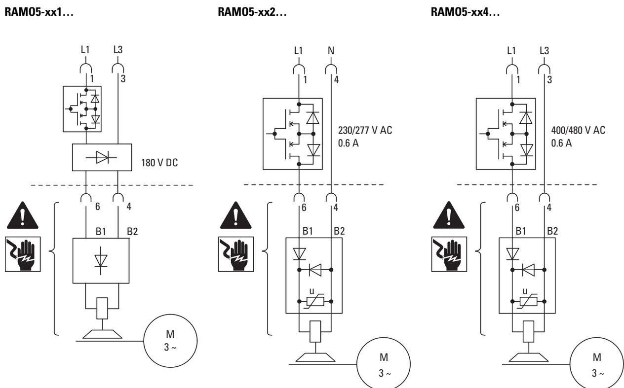
Figure 34: Control of the external brake with 180 V DC, 230 V AC/277 V AC and 400 V AC/480 V AC
