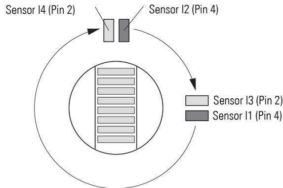
Figure 97: Example of clockwise rotary table control
