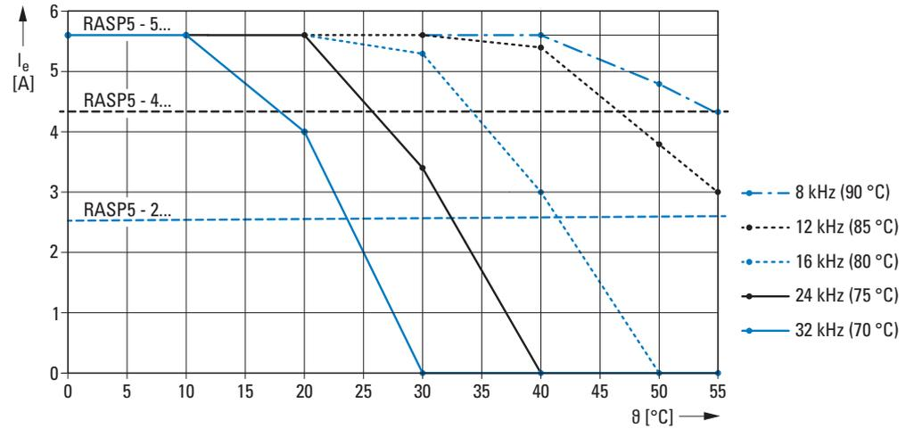
Figure 92:  $f_{PWM}$  = 8 - 32 kHz at RASP5-2..., RASP5-4..., RASP5-5...
