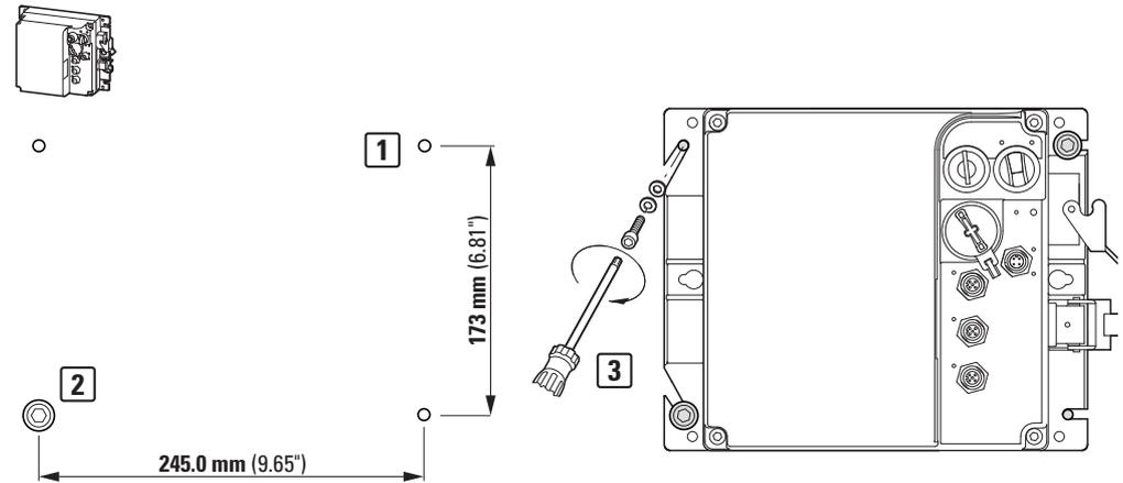
Figure 42: Fixing dimensions (standard) and mounting
