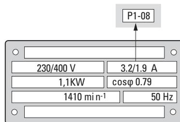
Figure 87: Set rated motor current
