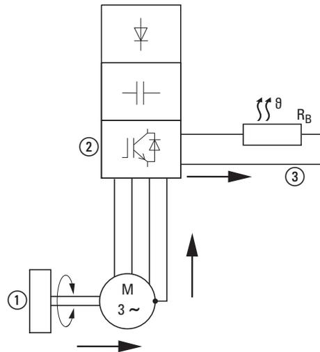
Figure 35: Regenerative braking with external braking resistance
