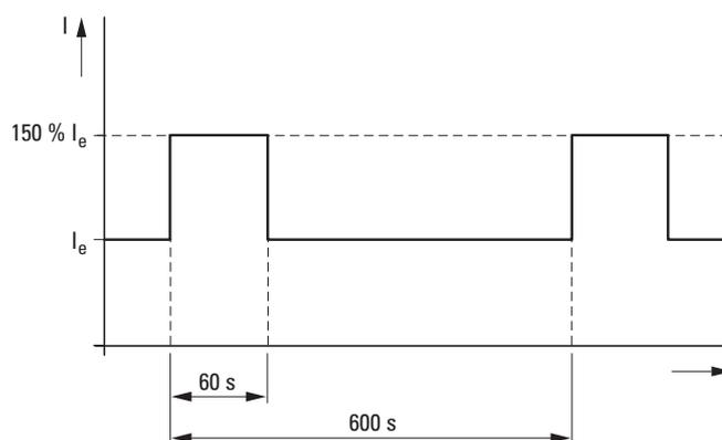
Figure 91: Overload cycle in operation
