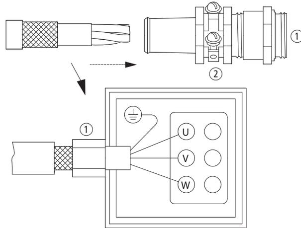
Figure 68: 360° screen contact at the motor terminal box
