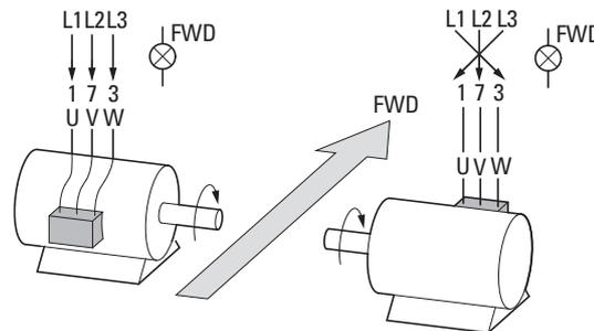
Figure 30: Example showing how to change the phase sequence
