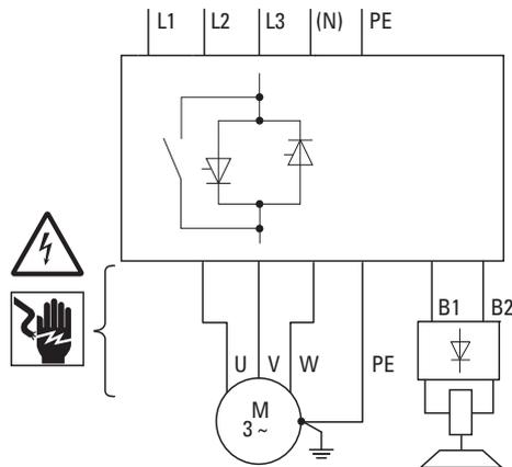
Figure 73: Direct starter with brake control RAMO5-Dxx1(2)(4)...RS1 (without repair switch)
