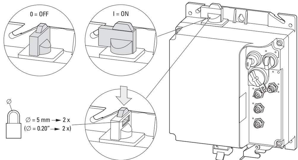
Figure 12: RAMO5 with repair and maintenance switch
