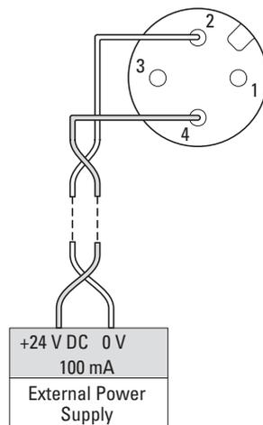
Figure 111: Connection example for quick stop
