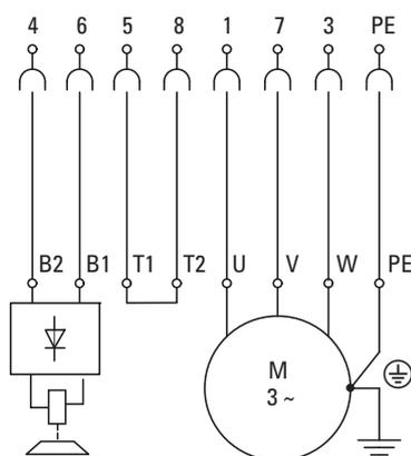
Figure 65: General connection with brake
