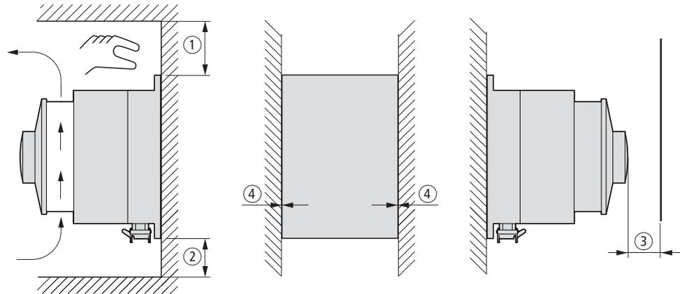
Figure 39: Clearances for thermal air cooling (example: RASP5)
