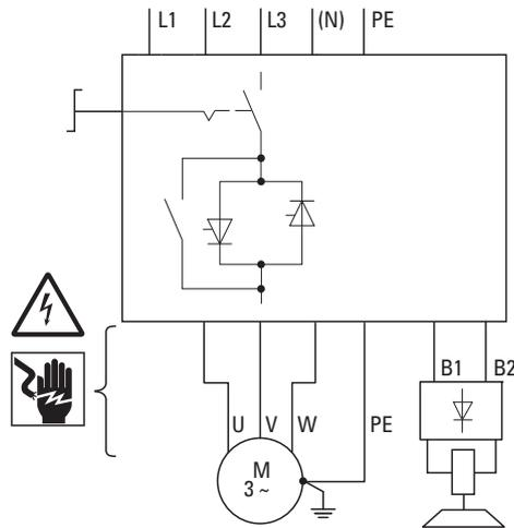
Figure 75: Direct starter with repair and maintenance switch and brake control RAMO5-Dxx1(2)(4)...RS1
