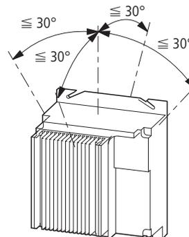
Figure 38: Mounting position of RASP5
