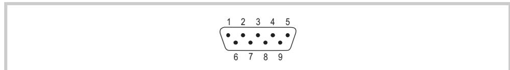
Abb. 17 CAN interface (9-pin, D-Sub, male, UNC)
