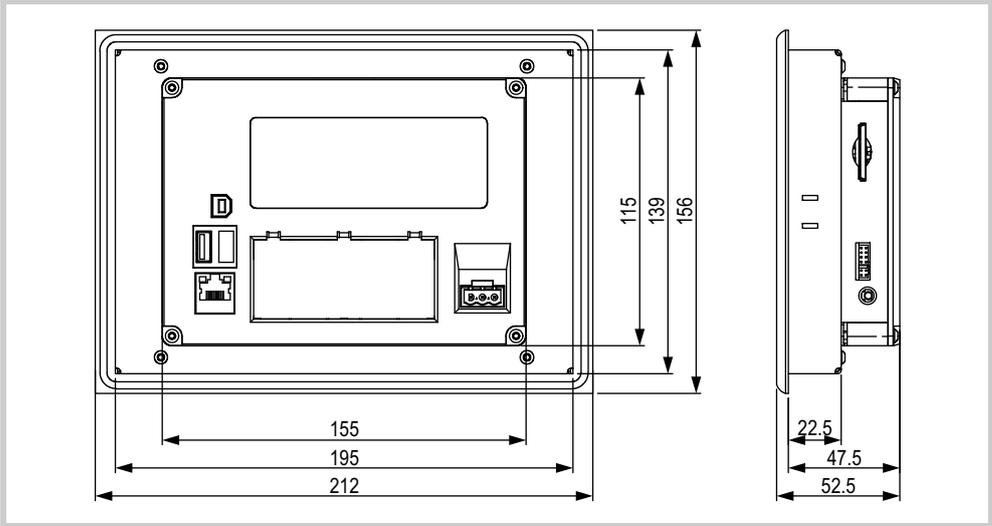
Abb. 31 Mechanical dimensions of the 5.7" devices in mm
