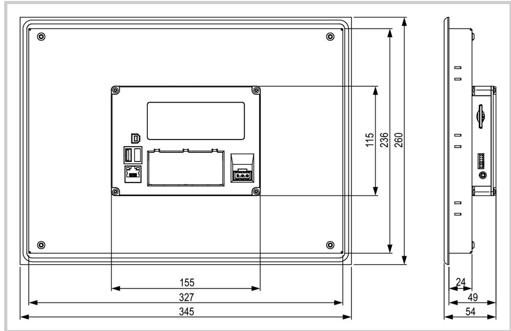
Abb. 33 Mechanical dimensions of the 10.4" devices in mm
