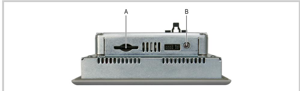
Abb. 3 Operating elements on the service side
