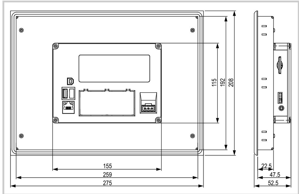
Abb. 32 Mechanical dimensions of the 8.4" devices in mm
