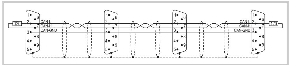
Abb. 18 Bus segment with four bus stations
