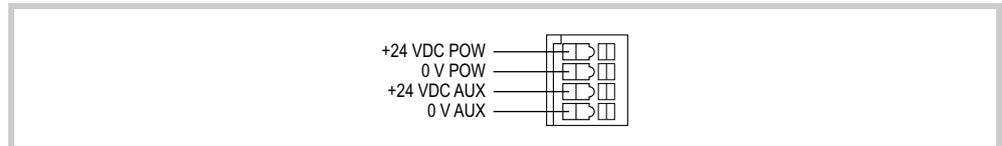
Abb. 15 WAGO connector (view from the wiring side)
