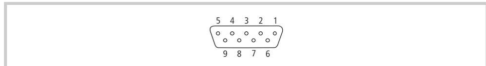
Abb. 19 Profibus interface (9-pin, D-Sub, female, UNC)
