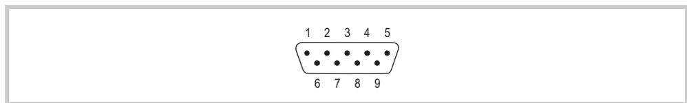
Abb. 21 RS485 interface (9-pin, D-Sub, male, UNC)
