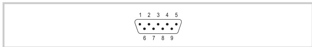
Abb. 9 RS232 interface (9-pin, D-Sub, male, UNC)
