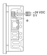
Abb. 11: Power supplied via plug connector
