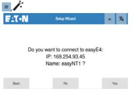
Abb. 43: Setup step 7 - directly establishing a connection
