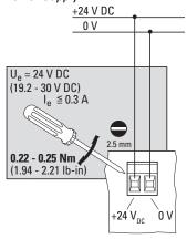
Abb. 10: Connecting the screw terminals on the plug connector
