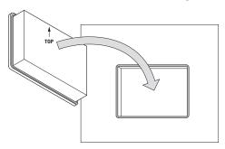
Abb. 8: Mounting in the installation cutout
