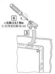
Abb. 9: Installing the holding brackets
