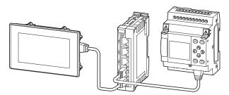
Abb. 55: Ethernet connection between the RTD and easyE4 devices through an Ethernet switch
