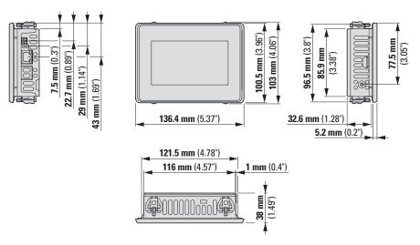
Abb. 57: Dimensions in mm (inches); tolerance: ±0.2 mm
