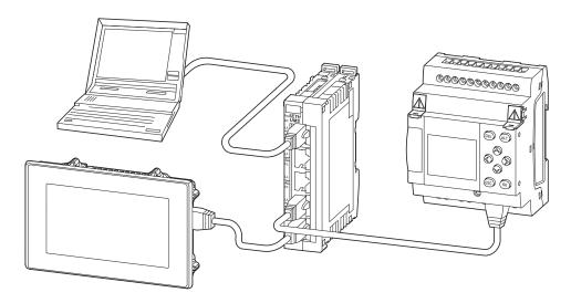
Abb. 56: Ethernet connection between the RTD and easyE4 devices through a switch with access to easySoft (PC)
