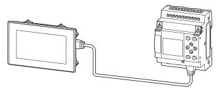
Abb. 49: Ethernet connection using the ports on the RTD and easyE4
