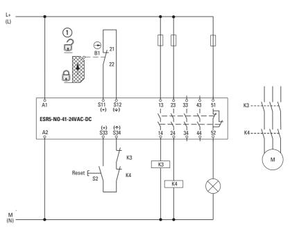
Figure 11:Single-channel safety door monitoring/manual start
