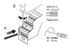
Figure 8: Connecting the cables
