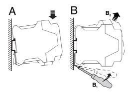
Figure 7: Mounting and removing
