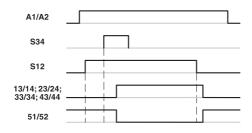
Figure 6: Time diagram for manual start
