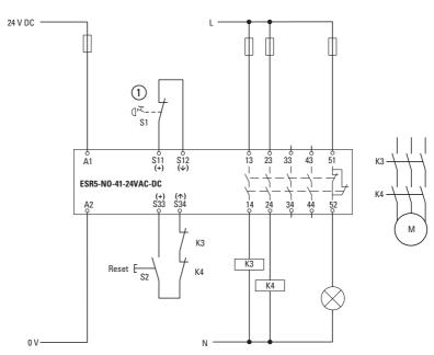
Figure 12:Single-channel emergency stop monitoring/manual start
