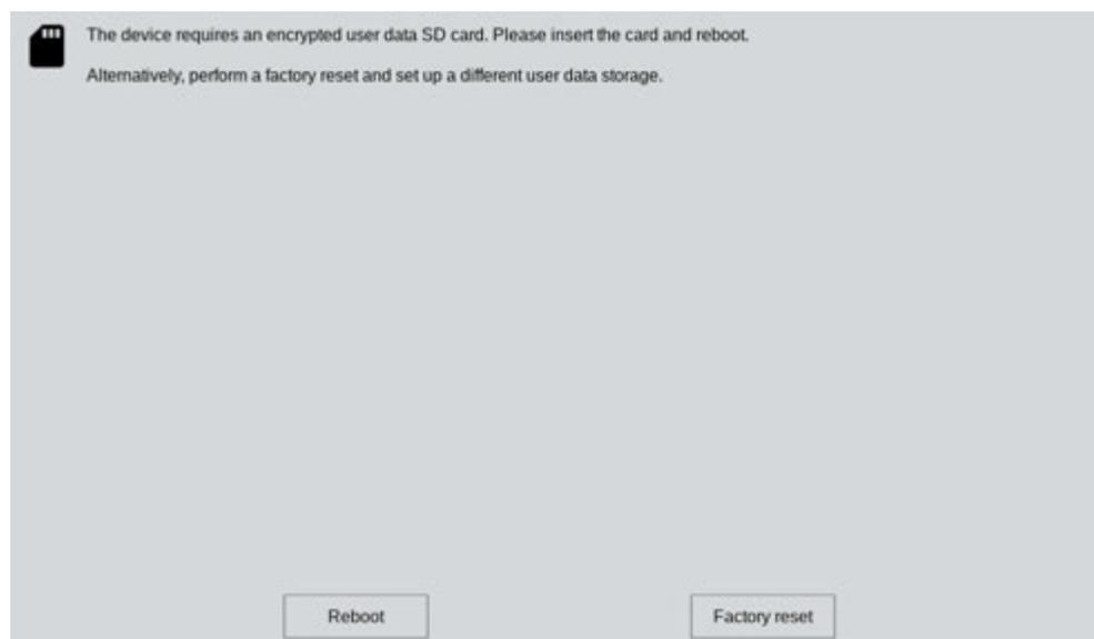
If this happens, either insert the correct SD card and restart the device by tapping **Reboot** or restore the device to its default settings by tapping **Factory reset**.
