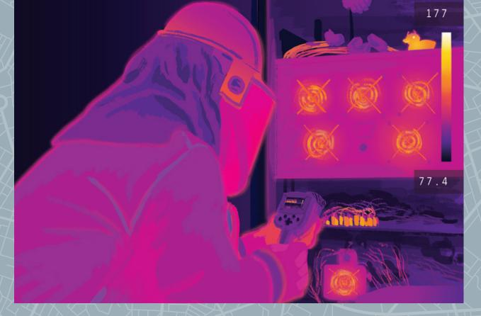
Once they arrived, Uncle Mike explained to Honey that he would use an infrared scanner to complete a thermographic inspection of the UPS.
