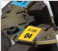
Color coded tabs on the die cage
