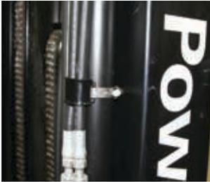
Good clamps can be inexpensive, yet highly effective for high-pressure surge lines. Anticipate and plan for a possible length change ranging from an increase of two percent to a decrease of four percent for high-pressure lines.
