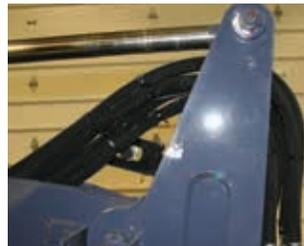
To achieve this, the hose should be positioned to bend like a hinge. Otherwise, the hose may have a tendency to take an S-bend, which is most likely to happen when the hose is pushed rather than bent. An S-bend installation results in excessive hose movement and reduced service life.
