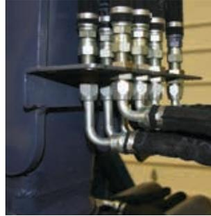
High-pressure hose must be routed to flex in only one plane. If plumbing requires that hose be routed through a compound bend, the hose should be "broken" into two or more sections so each will flex through only one plane. A spring guard will keep hose from bending beyond the minimum bend radius at the fitting, but it will not prevent the hose from twisting.
