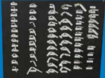
Nipple bending up to size -32 (DN51) for high-pressure spiral-hose assemblies
