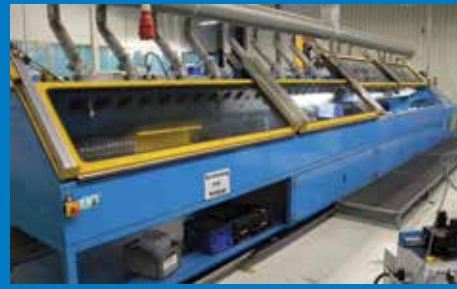
Proof testing of low- and high-pressure hose assemblies
